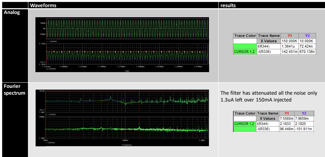
Figure 5.16: DC/DC Boost converter Input current conducted susceptibility simulation results for 150mA injection at 150kHz.
