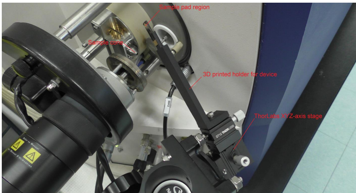
Figure 3.4. Image of a second version of the probe holder. A 3D-printed probe holder was coupled to a commercial ThorLabs platform for better probe positioning and more reproducible desorption and coupling to the MS inlet.
