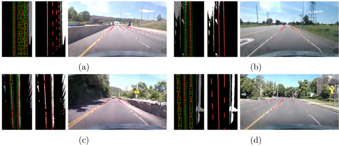
Figure 3.36: Examples of correct detections on straight line markings in different road environment: a major (3.36a) and secondary (3.36b) highway, a rural road (3.36c) and an urban road (3.36d). We notice how it is impossible in some cases to retrieve all the lines in the scene because of the limitation of field of view used to compute the BEV image. We point out however that all the lines within the ROI are clearly detected without outliers, regardless of the conditions of the road or the type of line (solid or broken).
