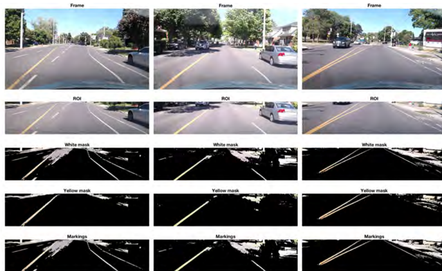
Figure 3.27: Final results of our pipeline on urban roads. The algorithm detects most of the interesting features, although some noise is created by tree shadows and other vehicles. Notice that some noise is also present outside the pavement, but that such cases are not relevant for our analysis as they can be removed in subsequent steps. Indeed, geometric considerations can be used to estimate their position as external to the road.
