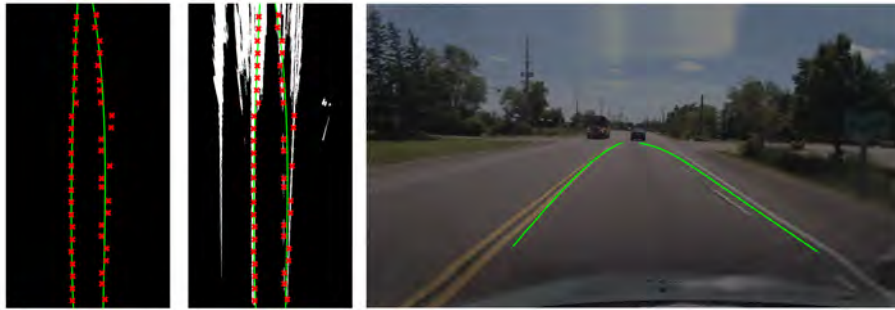
Figure 3.49: The behavior of polynomial lines in presence of outliers (false detections on the right side of the road): the model is not able to distinguish in- and out-lier points and fits them all.
