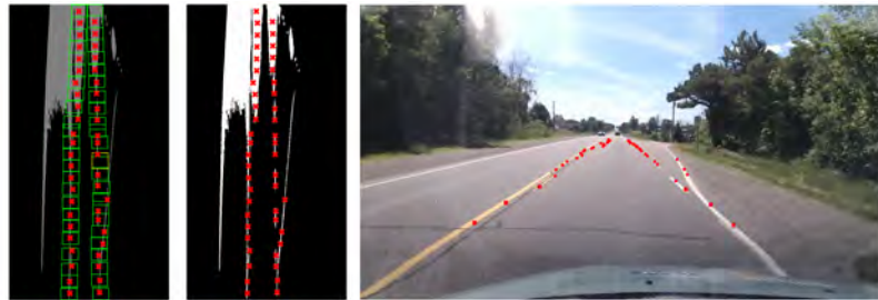
Figure 3.41: An unsolved issue in presence of lane splits delimited by broken lines is here depicted. Parts of the wrong branch are selected when the window overlaps only one of the branches at a time. As a result, outliers are produced despite the adjustment described in Section 3.4.3. We must point out also how in this example it is only for our luck that the tracking has continued on the correct line, but that in principle once this alternating behavior is triggered any of the two lines could be followed at last, producing potentially wrong results.
