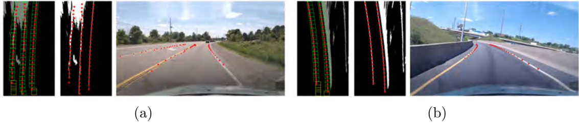
Figure 3.37: The results produced by the algorithm on smooth road bends. The windows are large to follow the lines adequately but also small enough to avoid the introduction of outliers. A bit of noise is present however in the distance, but for an illumination effect completely uncorrelated to the road bend.
