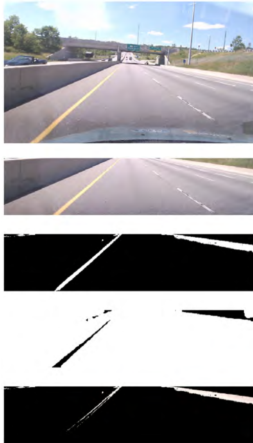
Figure 3.23: Pipeline for the correction of the yellow mask by morphological by usage of a road mask. In order, the following are shown: the original frame, our ROI, Y_w , the road mask R and finally the original frame filtered by Y_w \odot R . We notice how this technique is not particularly effective due to the removal of the yellow markings in the road mask. It results very hard to cope with this issue without opening too much the road mask.
