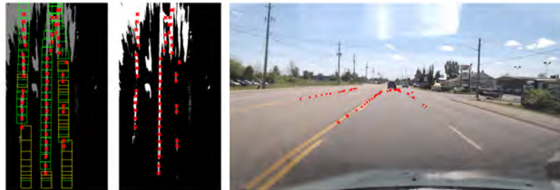
Figure 3.39: Noisy detections and outliers are formed in presence of severe noise in the feature image itself. This is a sign that although the algorithm can improve many situations in which some impurities are present, it cannot cope with them where their level is too high. We notice however that this phenomena occur mostly on the far end of the lines, and that therefore could be avoided considering a shorter ROI.
