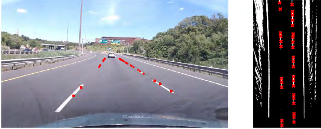
Figure 3.33: A projection on the front view image of the retrieved points seen also in Figure 3.32. Notice how well they adhere to the line markings of the ego-lane.
