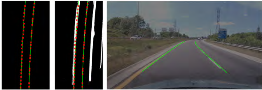
Figure 3.47: Example of the satisfactory performances of a quadratic model in presence of a road bend.
