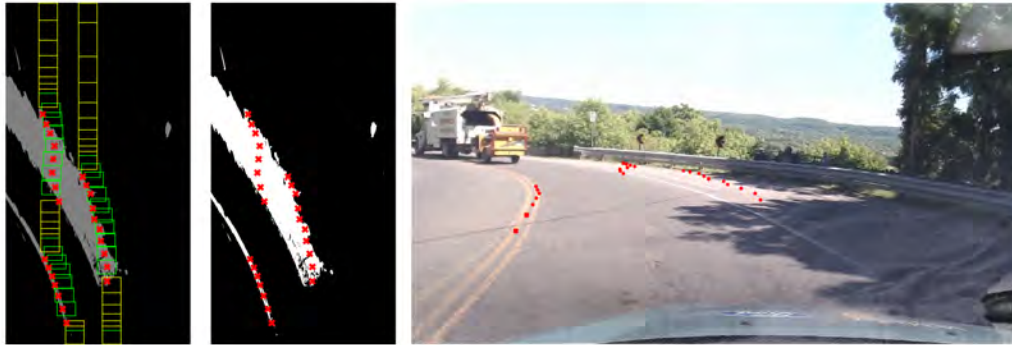
Figure 3.38: The poor performances of the algorithm in case of a sharp bend in the road, such as a hairpin turn. The windows are not large enough to detect a new candidate on the inner line of the curve and a completely wrong detection is returned. Results of this kind must be avoided or prevented also for the high risks that recognizing a turn as a straight lane might determine.
