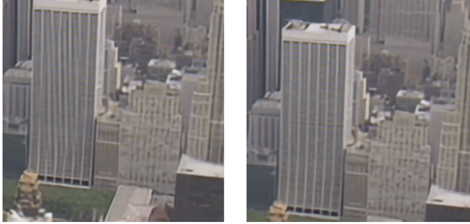
Figure 4.1: Left: smaller patches combined output Right: larger patches combined output. From PSNR scores perspective the left side even slightly larger than the right side, but there is the artificial effect on windows of the building. The upscaling factor is set to 4.
