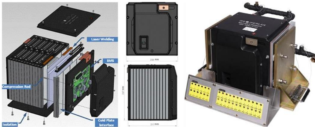
**Figure 6.1.** Design of a battery module and the resulting prototype investigating the thermal management of high-power cells [99].
