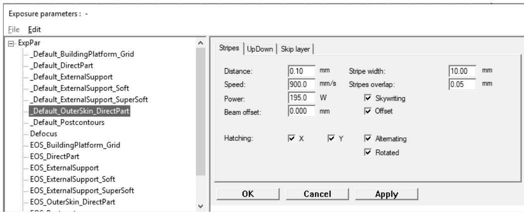
Figure 18: Additive manufacturing software parameters - strips
