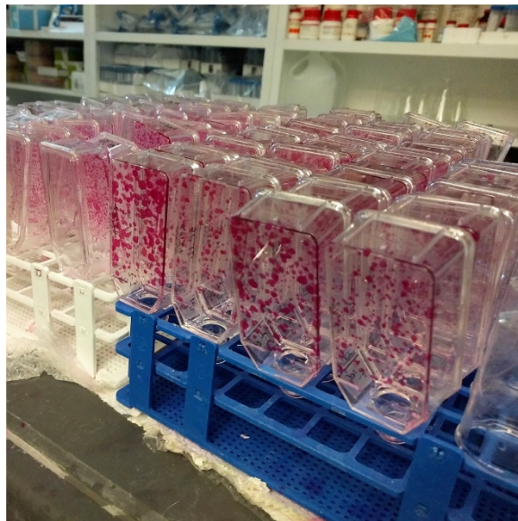
Figure 1 – Following staining using diluted Fuchsin-Carbol, colonies with more than 50 cells are distinctly visible allowing for counting without the use of a microscope
