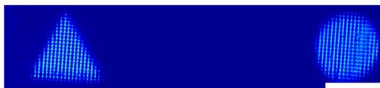
**Figure S2.28.** Simultaneous image collection transmission of two objects from the WEL-3<sub>(-30°, 0°, 30°)</sub> lattices. Scale bar = 1 mm.
