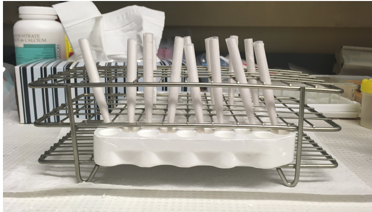
Figure 3.1: 15 ‘bones’ were made; they are Plaster of Paris (PoP) with a specific Pb concentration (0 ppm, 50 ppm or 150 ppm). Each of them was cut and kept to a length of 37 mm for consistency.
