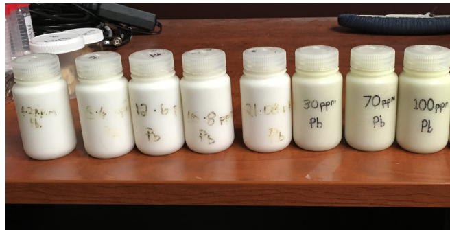
Figure 1.12: A series of phantoms in different lead concentrations.
