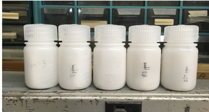
Figure 3.3: 5 mouse-mimicking bone Pb phantoms were prepared with and average concentrations of 0, 16.67, 33.33 and 50 ppm respectively.
