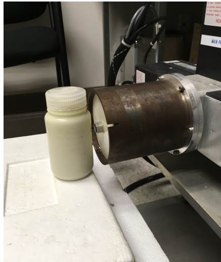
Figure 1.9: A close-up of the existing bone lead phantom measurement.
