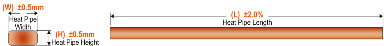
Figure 5.7: Flat heat-pipe dimensions guide [65]
