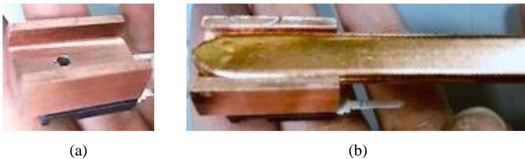
Figure 6.10.a: A groove with the same width as the heat pipe is machined on one side of the copper block, b: the heat pipe is slid inside the groove
