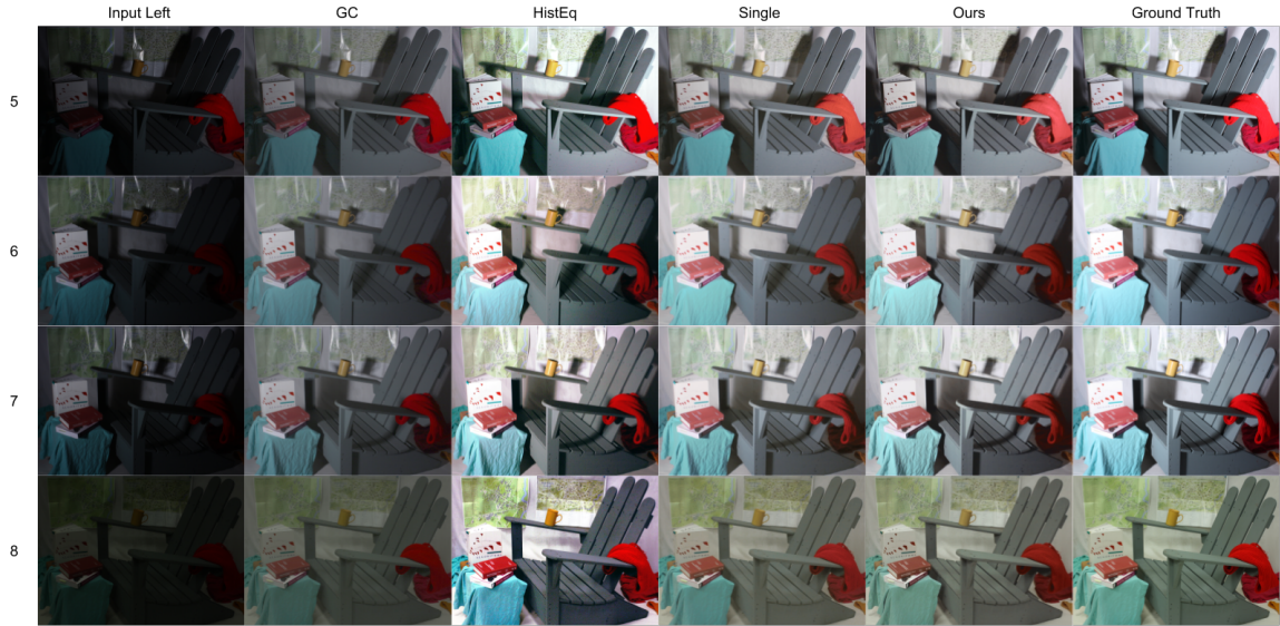
Figure 4.12: Results for different methods compare to our method. Gamma correction (GC) with \lambda = 0.5 , Histogram equalization (HistEq), Single left image (Single), Ours.
