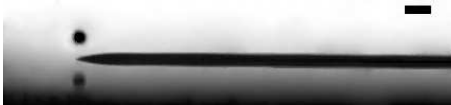
(c) Size of the gap between the deposited droplets = 73\ \mu\text{m} .
