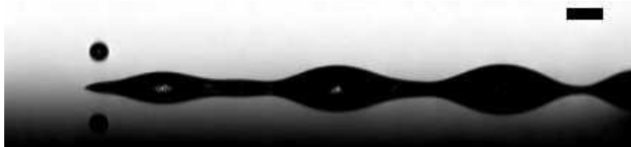
(d) Size of the gap between the deposited droplets = 28\ \mu\text{m} .
