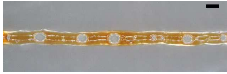
(a) Size of the gap between the deposited droplets = 73 \mu\text{m} .
