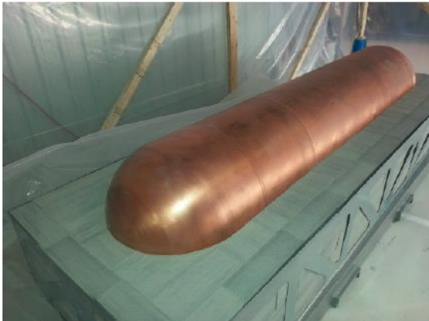
Figure 1.5: UFC inside HCB clay block (Gierszewski, 2018).
