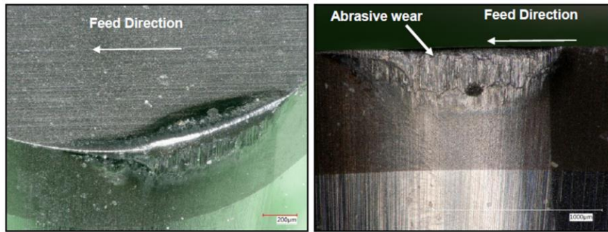
Optical images of CBN cutting tool with composition 3 after cutting length of 29565 m
