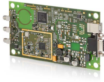
Figure 5.1 RFID reader implemented in hybrid RFID doorway IPS.[1]
