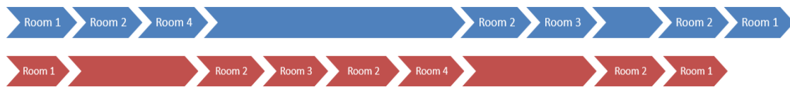
Figure 4.16 (A) The trajectory of two participants walking through a residential apartment equipped with three hybrid BLE doorway monitoring systems. The trajectory was used to evaluate the IPS’s accuracy for monitoring the position of multiple occupants within multiple rooms. (B) The order in which each participant crossed through a doorway.
