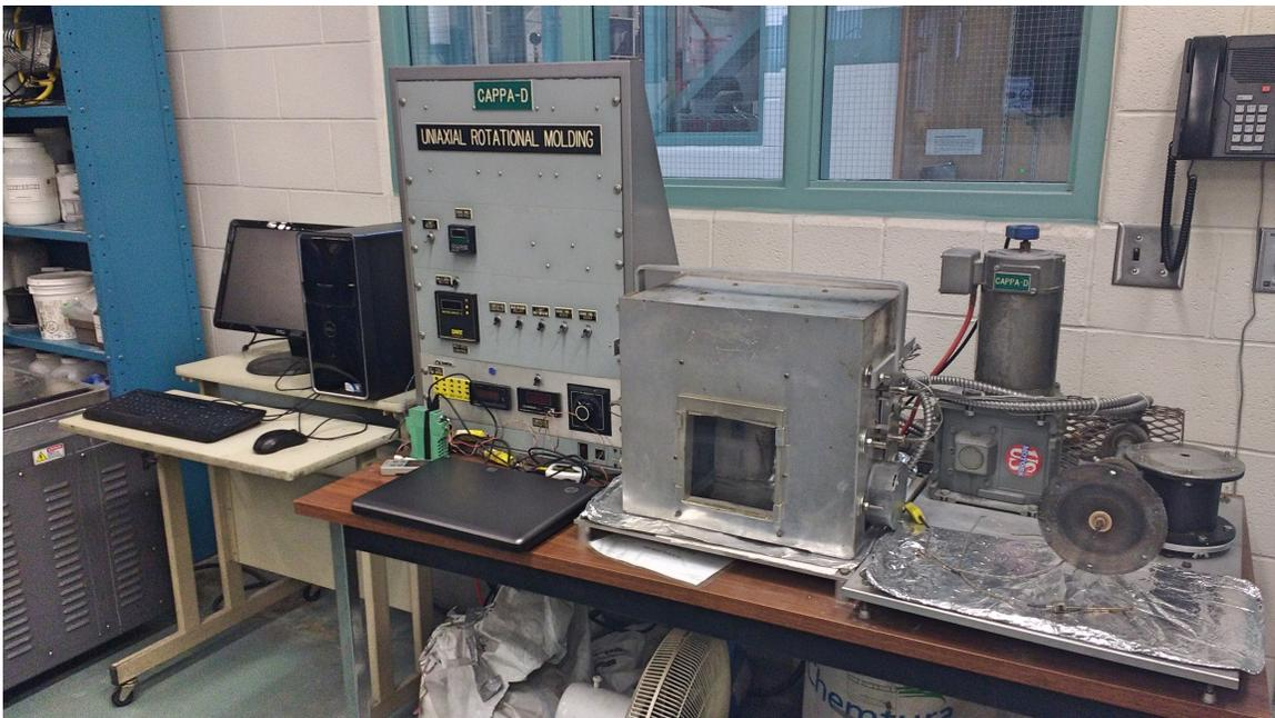
Figure 5.22: Experimental setup for rotational molding
