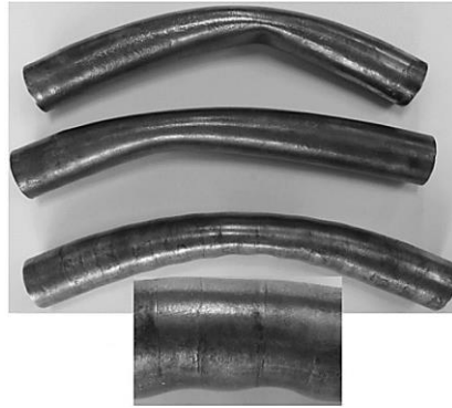
Figure 1.5: Bending behavior of different tube specimens: Normal steel (top), fully carburized (middle), composite tube (bottom) [25]
