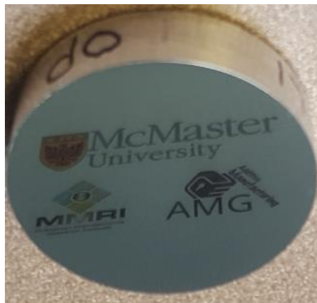
Figure 6.11 The ultra-precision machined surface of the additively manufactured Al mirror.
