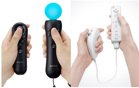
Figure 2.5: Nintendo’s Wii Remote and Playstation Move Controllers with Joystick accessories
