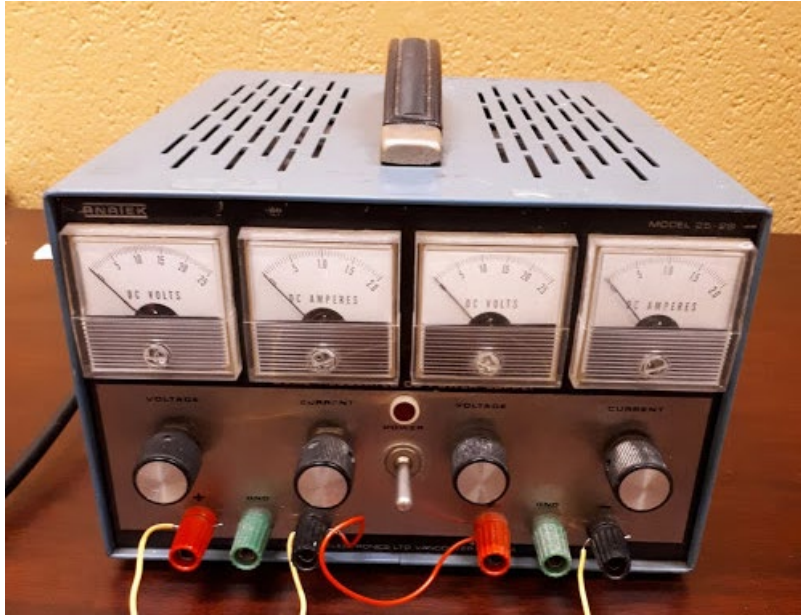
Figure 18: Anatek Model 24-2D Power Supply
