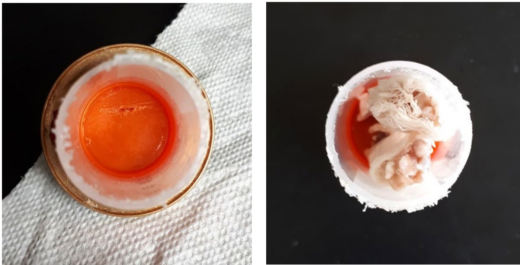
Figure 56: Left – sample holder with etched marking. Right – leg bones wrapped in gauze placed in the sample holder (right leg bones are on top of the marking).
