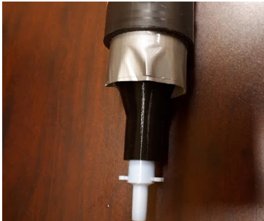
Figure 46: Portion of the tube showing the input adapter inserted
