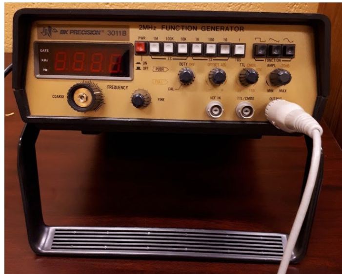
Figure 26: BK Precision Model 3011B signal generator
