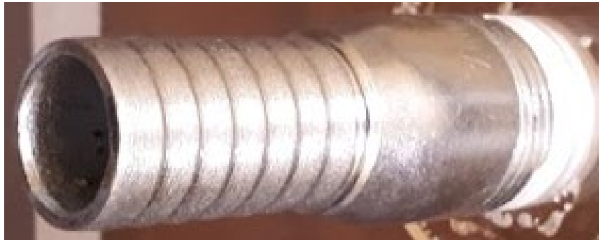
Figure 38: \frac{3}{4} ” barbed fitting attached to the box
