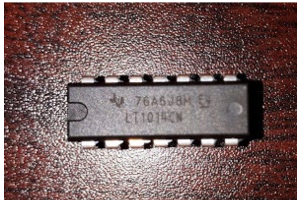
Figure 17: LT1014CN integrated circuit
