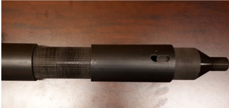
Figure 48: Portion of the tube showing flow restrictor and scavenging rate control hole
