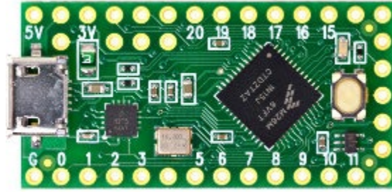
Figure 12: Teensy LC Microcontroller
