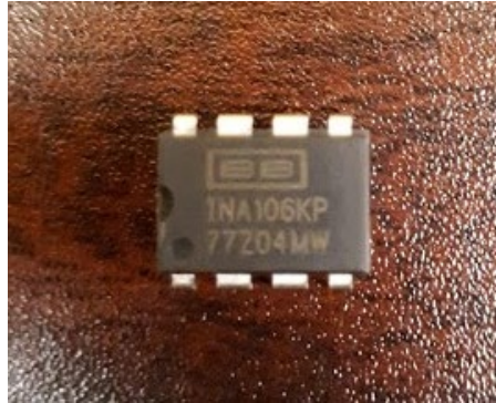
Figure 19: INA106KP integrated circuit
