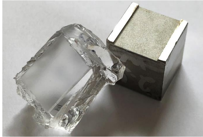
Fig. 3.1.4 An EDM textured surface with its PDMS casted surface.
