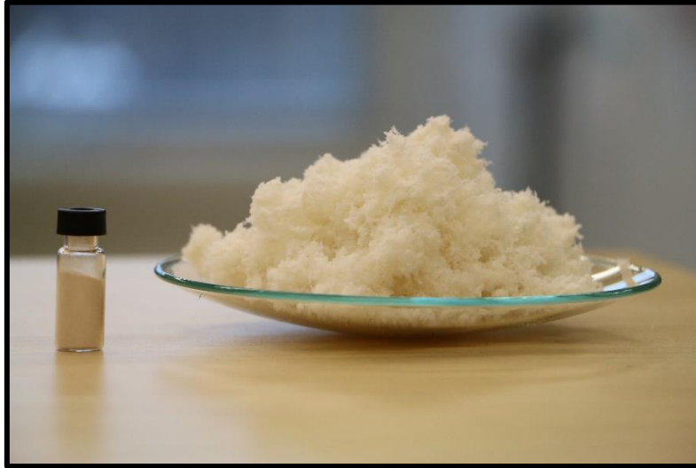
Figure 11. Photograph comparing the same mass of pectin before and after the PGX process
