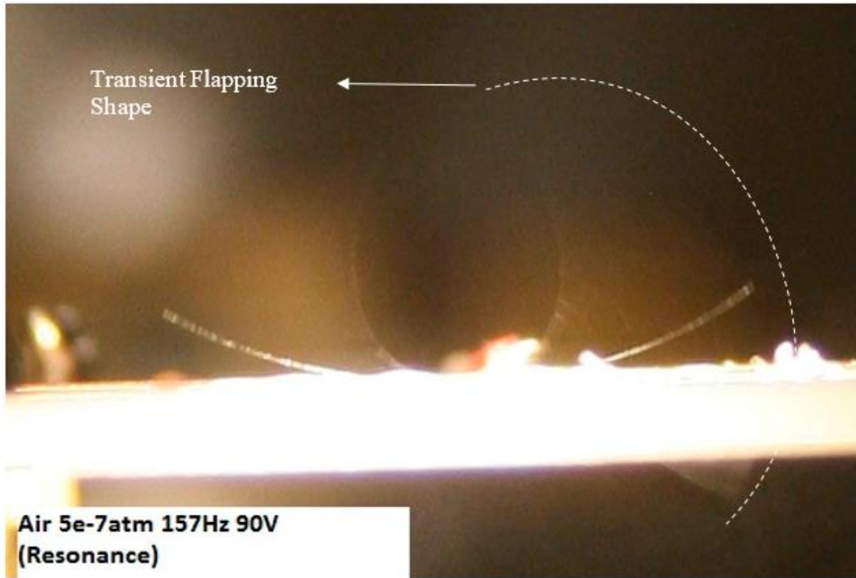
Figure 57: Wings at resonance show very large A_r when wing actuated at 90V, 157Hz in vacuum.
