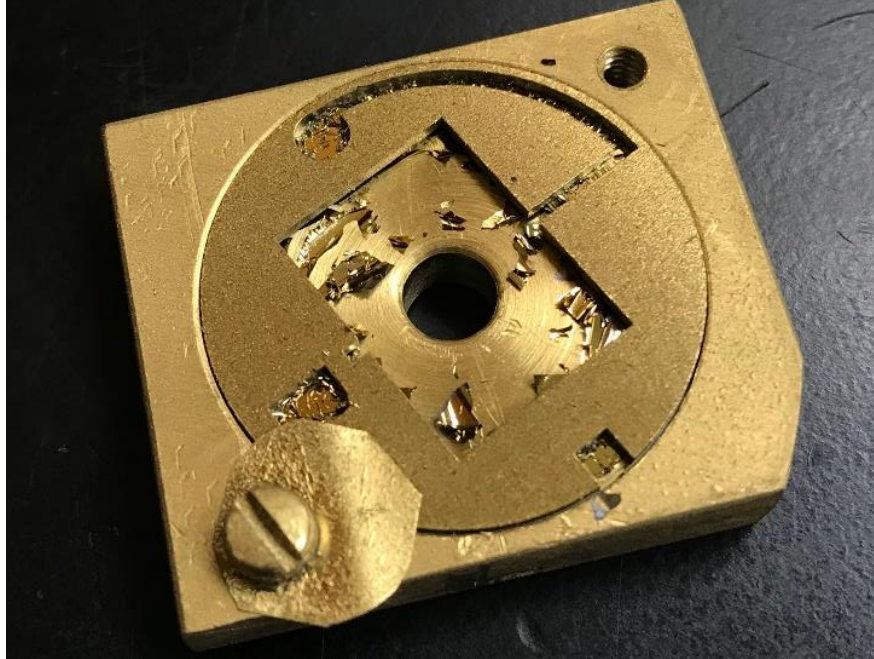
Figure 60: Shattered sample after Mo and Au deposition. The rest of the sample is covered by the shadow mask and both are held in place by a sample holder.
