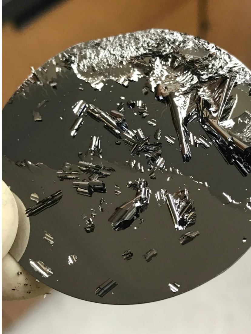
Figure 61: Result of sputtering Molybdenum on a Silicon wafer using the new 'optimal' sputtering parameters. The delamination continued to occur after taking the sample out of the chamber.
