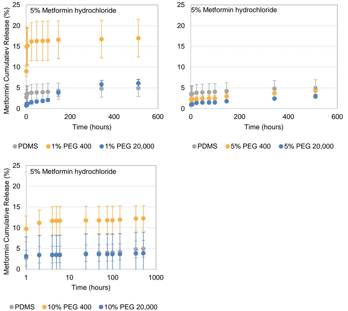
Figure 5.9. Release of metformin hydrochloride does not significantly differ in the presence of PEG<sub>400</sub> or PEG<sub>20,000</sub> in comparison to PDMS-only control. 1% PEG<sub>400</sub> showed statistically significant difference, however this value looks to be an outlier due to a larger variation between experimental replicates.
