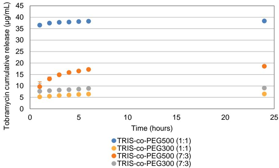
Figure 4.16. Release of tobramycin from silicone hydrogels, measured over 24 hours (stdev, n=4).
