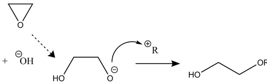
Figure 2.12. Polymerization of ethylene oxide.
