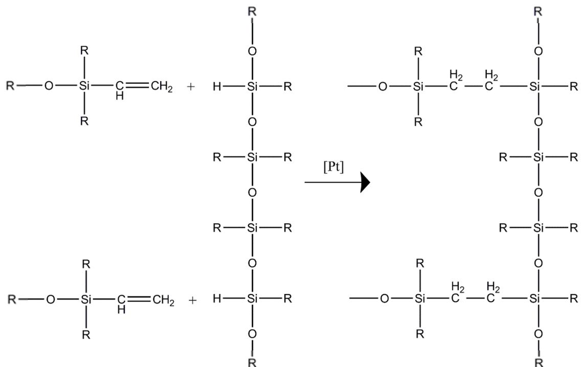
Figure 2.10. Platinum based polymerization / crosslinking of silicones.
