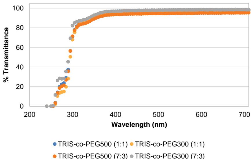
Figure 4.9. The light transmittance of each material across the UV and visible spectrums ( $n=3$ ).
