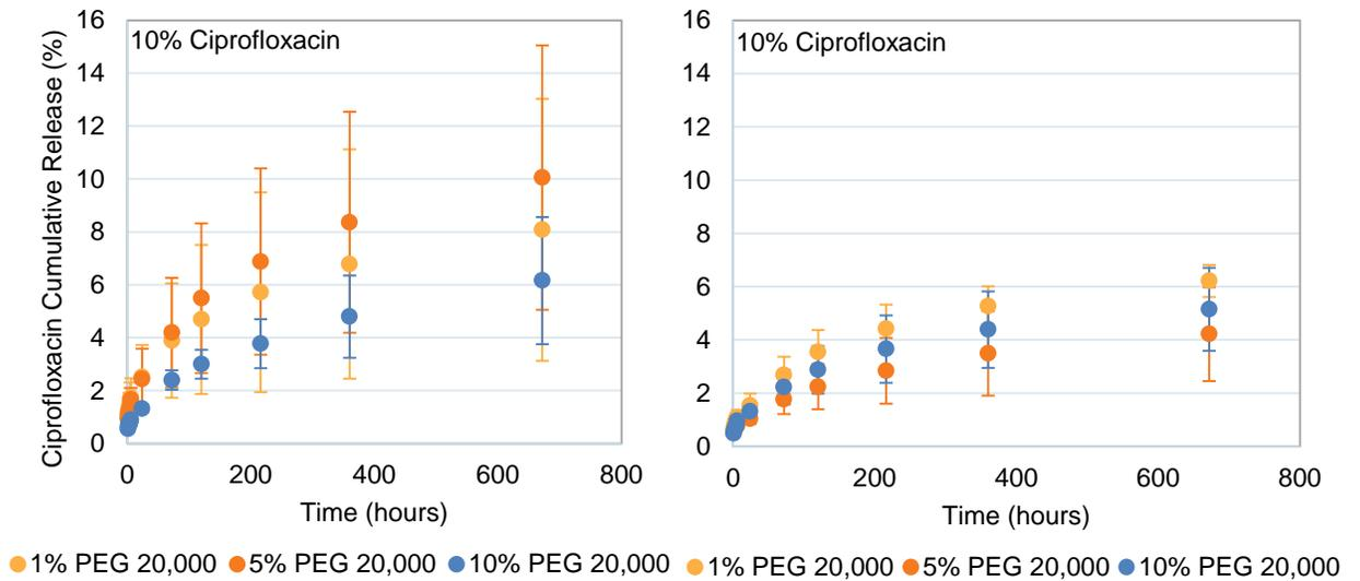
Figure 5.4. Effects of increasing PEG<sub>20,000</sub> concentration on ciprofloxacin release. Data indicate the release curves are not statistically significant.
