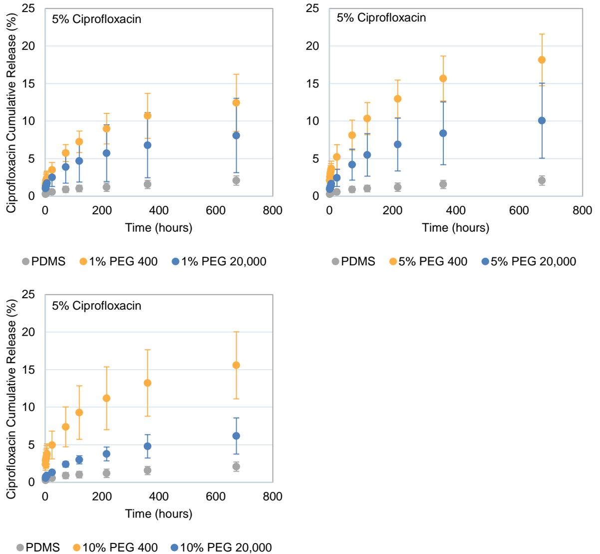
Figure 5.1. Cumulative release of ciprofloxacin loaded at 5% in PEG<sub>400</sub> is statistically significantly greater than PDMS at all PEG concentrations tested. Release from materials containing PEG<sub>20,000</sub> was only statistically different from PDMS with 10% PEG<sub>20,000</sub>.
