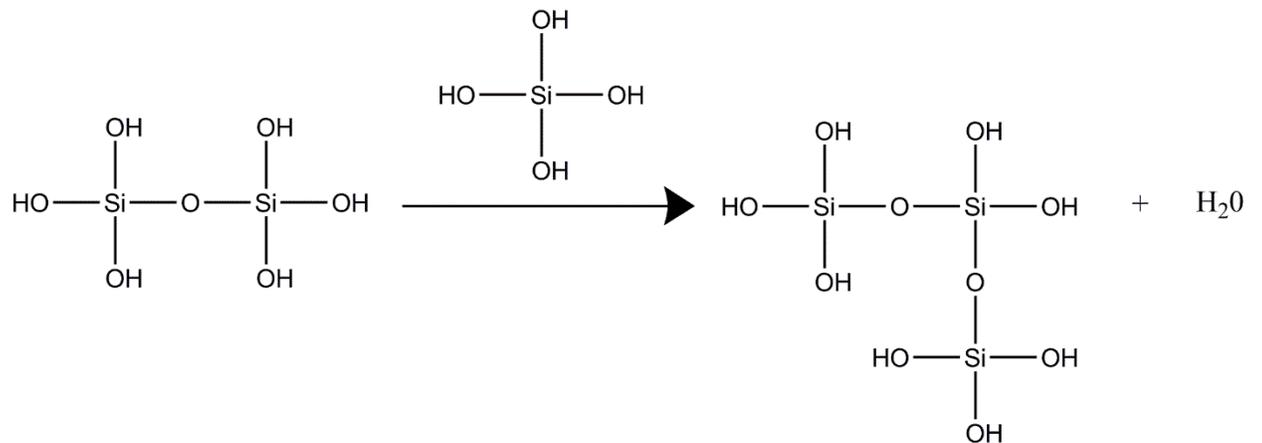
Figure 2.9. Polymerization of silicones.
