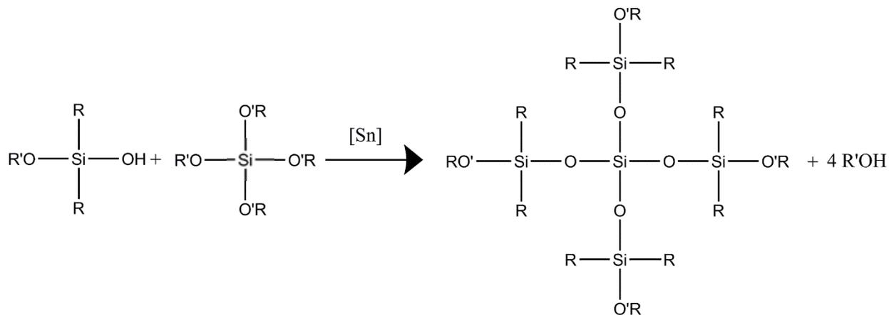
Figure 2.11. Tin-based polymerization / crosslinking mechanism of silicones.
