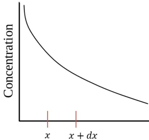
Figure 2.2. Flux of a molecule moving from a location of high concentration to low concentration.
