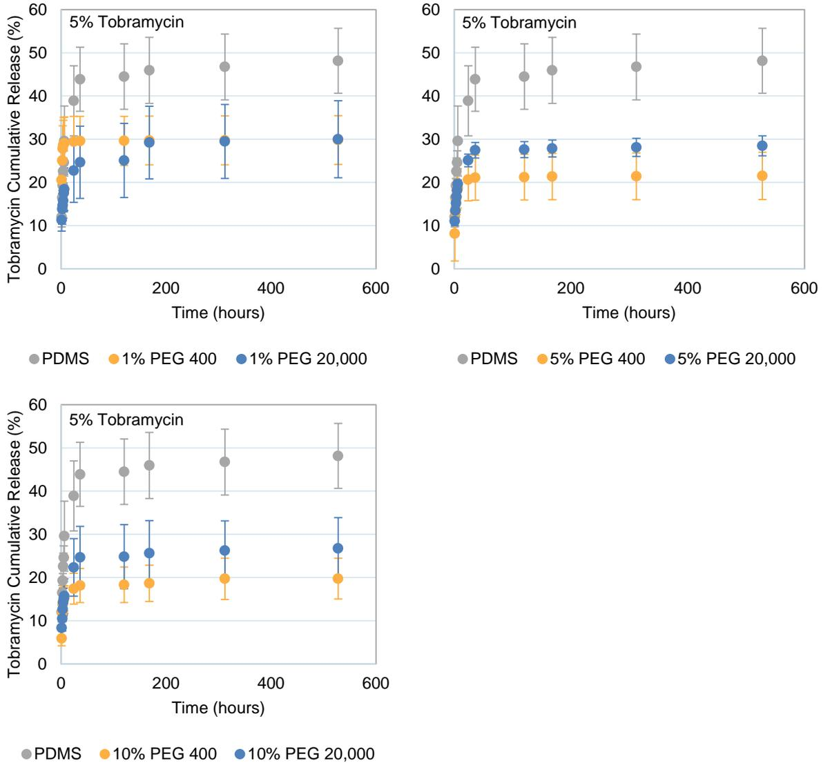
Figure 5.5. The presence of PEG<sub>400</sub> or PEG<sub>20,000</sub> statistically significantly reduces tobramycin drug release in comparison to PDMS-only discs.
