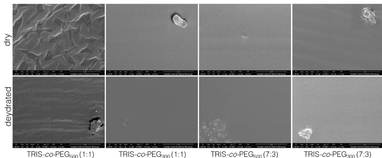
Figure 4.5. Surface morphologies of TRIS-co-PEG materials as observed using SEM. Representative images shown are taken at 25,000x magnification.
