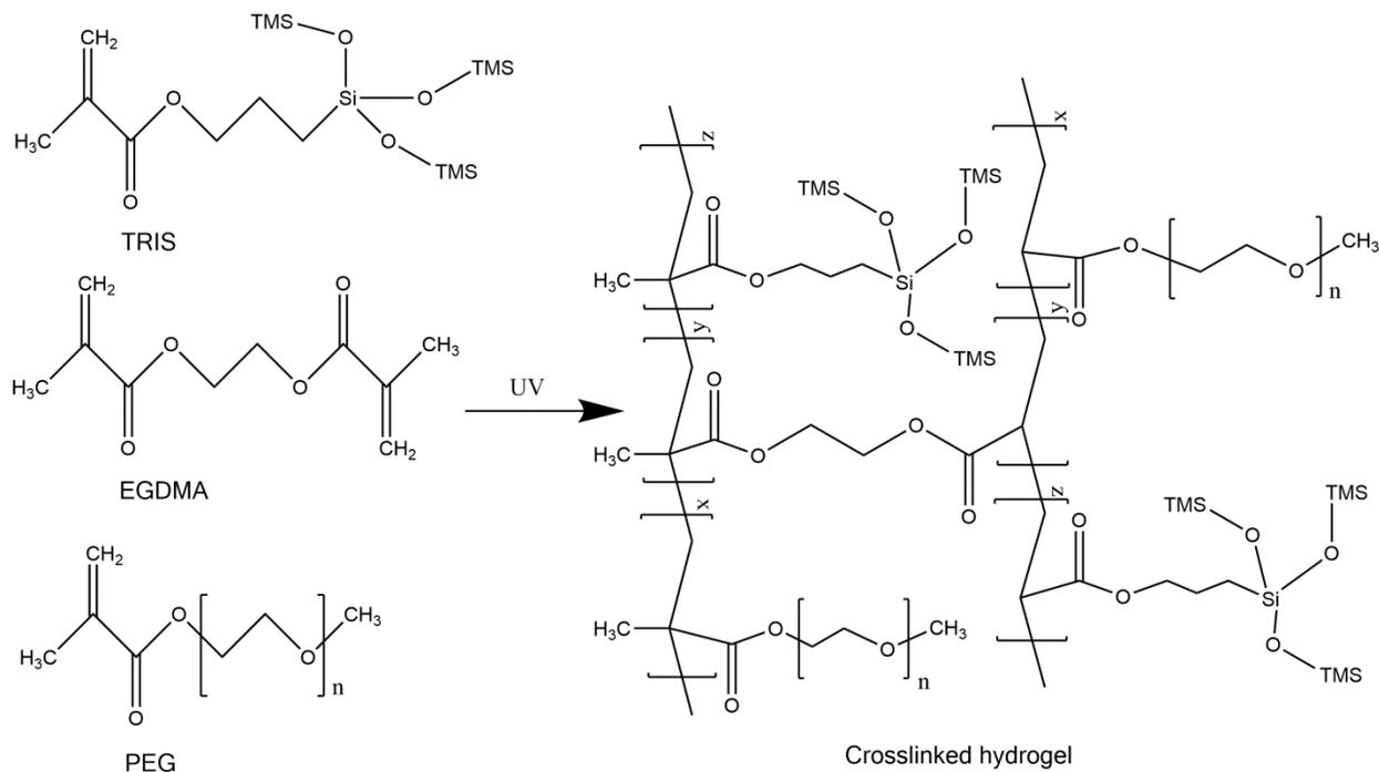
Figure 4.2. Schematic depicting the reaction between macromers and crosslinker to form the novel hydrogel materials.  $n$ : repeating ethylene oxide units corresponding to 300 or 500 molecular weight PEGs.  $x, y, z$ : varying macromer ratios that exist within the hydrogels. TMS: trimethylsiloxane
