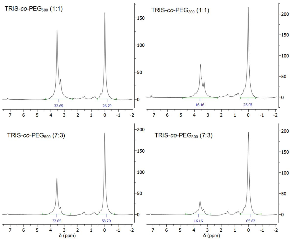
Figure S14.2. Hydrogel <sup>1</sup>H NMR spectrums. Hydrogels were solvated in CDL3. Identifying peaks were integrated only. Refer to Results for analysis.
