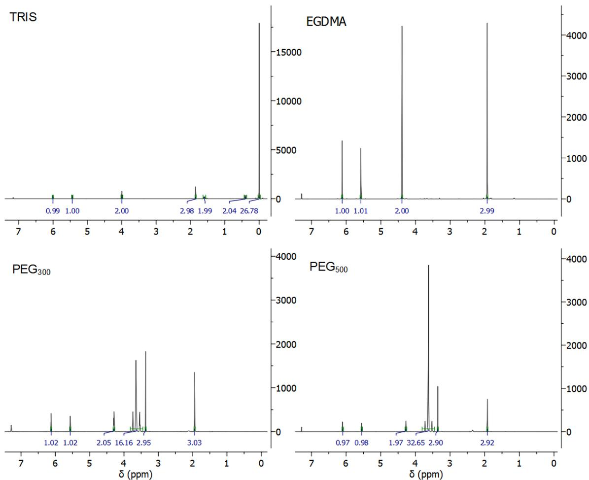
Figure SI4.1. Macromer <sup>1</sup>H NMR spectra. Macromers were solvated in CDL3. Refer to Results for analysis and peak identification.
