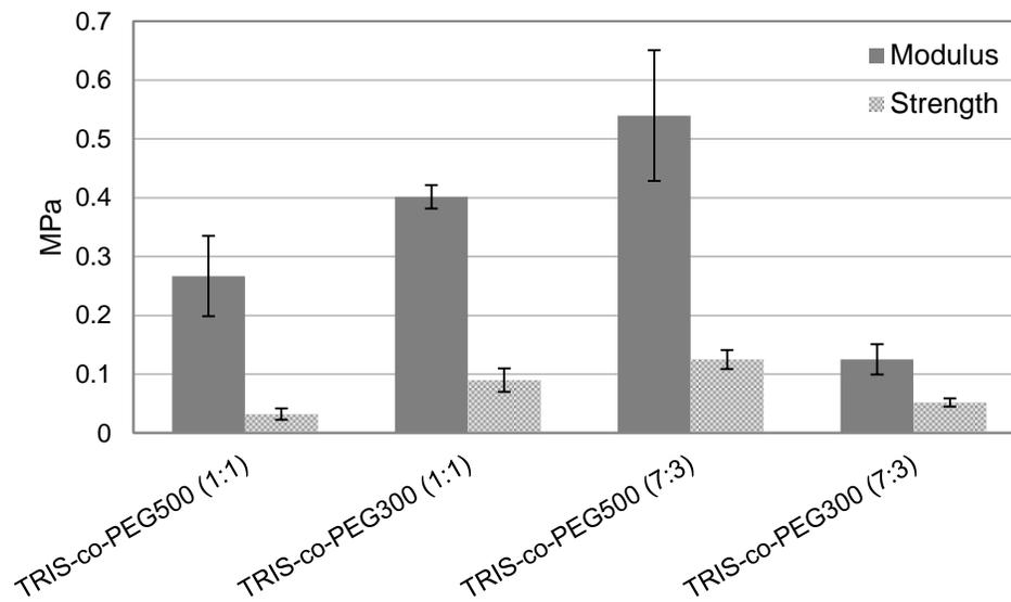
Figure 4.7. Mechanical properties of materials (stdev, n=4).
