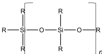
Figure 2.7. Standard molecular structure of silicones. R groups can represent varying side chains.
