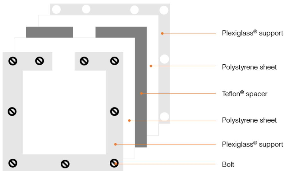
Figure 4.1. The hydrogel mold consisted of a 0.5mm Teflon® spacer placed between two polystyrene anti-static sheets. Thick Plexiglass® surrounded either side of the polystyrene sheets for physical support.
