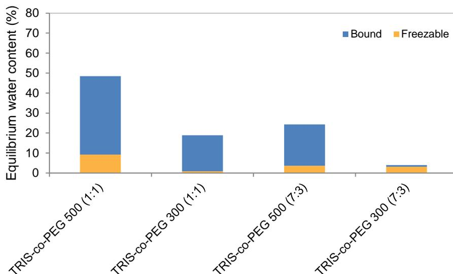
Figure 4.13. Correlation between the number of moles of ethylene oxide in each material and the corresponding equilibrium water content.
