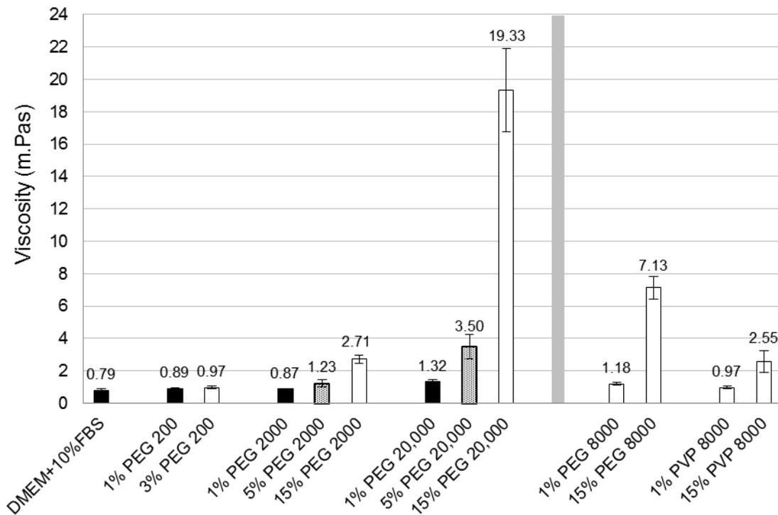
Figure 3.7. Viscosity of cell media with varying polymer molecular weights and concentrations. Precise average viscosity values are stated above each bar for ease of comparison. Error bars denote standard deviation ( $n=3$ ).
