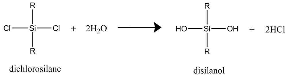
Figure 2.8. Hydrolysis of silanes to form silanols.
