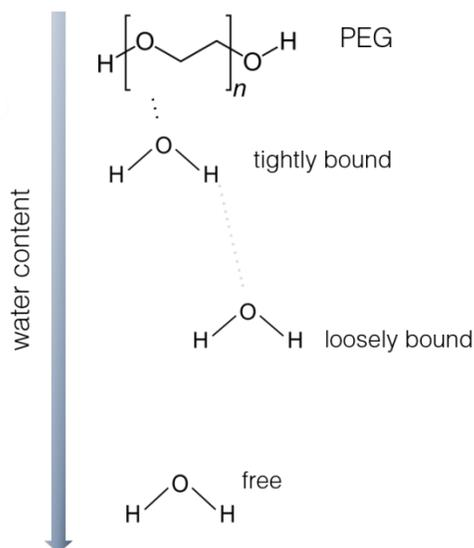
Figure A1. States of water in the presence of poly(ethylene glycol), with increasing water content. Image is adapted from Tranoudis et al [36].
