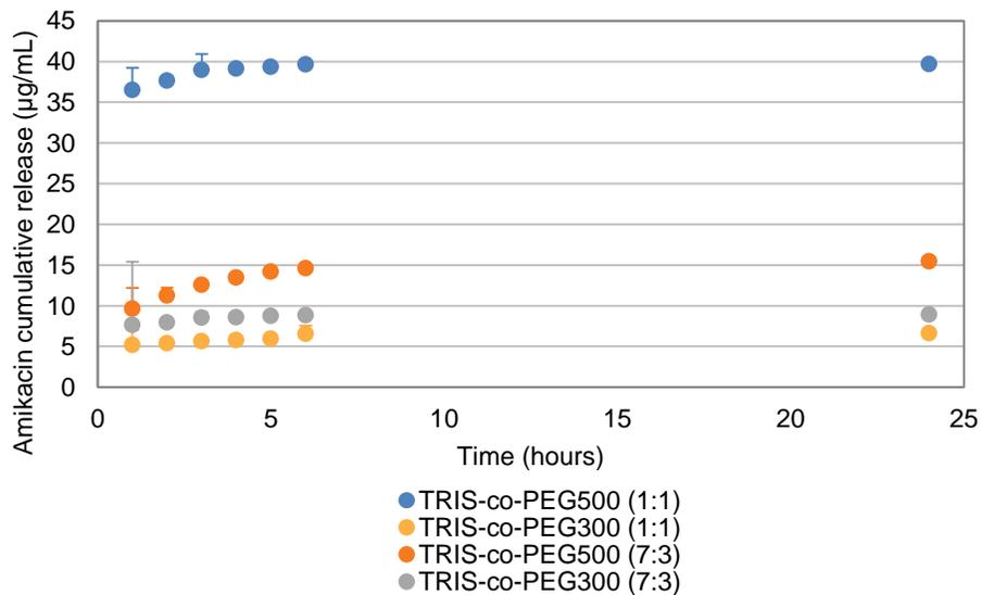
Figure 4.17. Release of amikacin from silicone hydrogels, measured over 24 hours (stdev, n=4).
