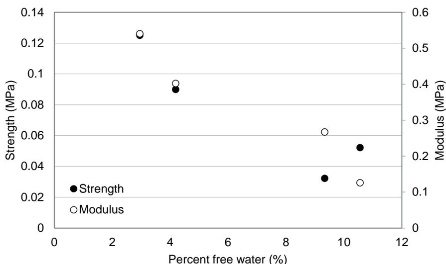
Figure 4.15. Relationship between the mechanical properties and amount of free water (% of EWC) in each hydrogel.
