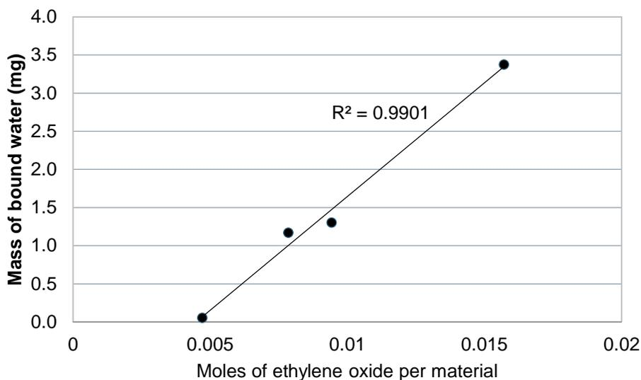
Figure 4.14. Relationship between the number of moles of ethylene oxide units and the amount of bound water.
