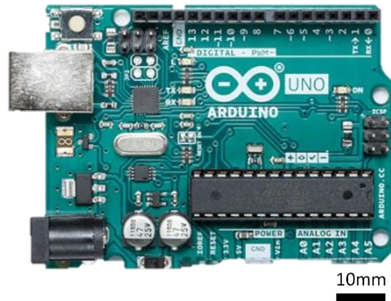
Figure 3.14: Picture of the Arduino Uno used in the prototypes that utilize a photodiode detection method
