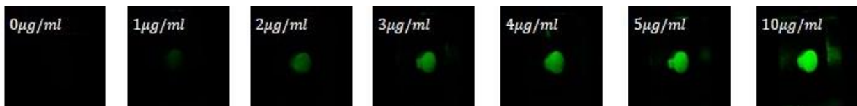
Figure 4.14: Experiment demonstrating \lambda - DNA characterization in Prototype 4 with the imaging prototype. Samples were loaded in the reservoir devices with increasing concentrations of \lambda - DNA to show the capability of the Sepsis Check to linearly characterize between \lambda - DNA concentration and optical intensity.
