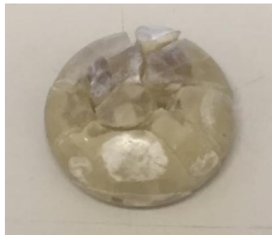
Figure 3.2 Solidified slag with precipitates on the surface
