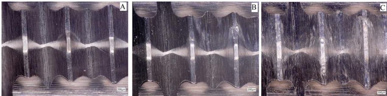
Figure 35 First three chamfered threads of uncoated roll form taps used with the (A) Hocut 795H, (B) SAC and (C)Sunflower oil
