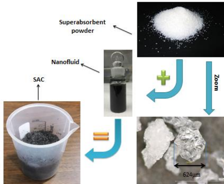
Figure 7 Sequence of the SAC preparation (polymer powder is mixed with a nanofluid, and after 10 min stabilization, SAC is ready for use.)
