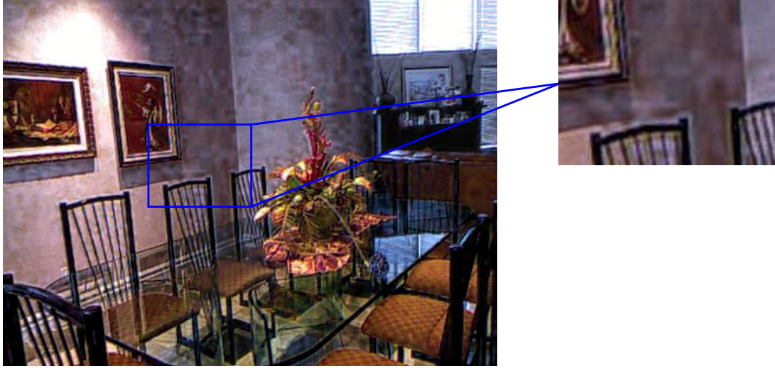
Figure 5.1: Example of block effect that occurs in indoor image.
