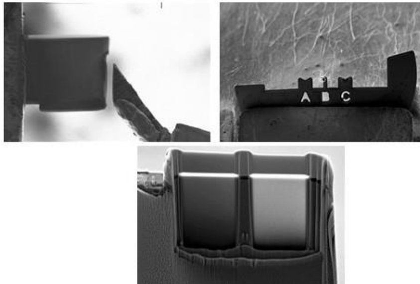
Fig 3.4. Top: Welding process for internal method. Bottom: Final TEM lamella.
