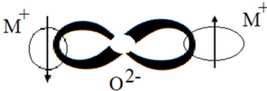
Fig. 2.3 Representation of a superexchange interaction in an oxide system.
