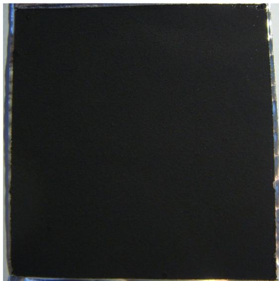
Figure 96: Successful coating of LFPO-CB on Aluminium
