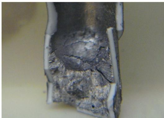
Figure 65: Autoclave sample A11. Elemental silicon and sodium were reacted to produce cylindrical NaSi slabs.
