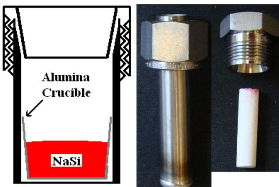
Figure 35: Swagelok® autoclave design, with long alumina crucible.
