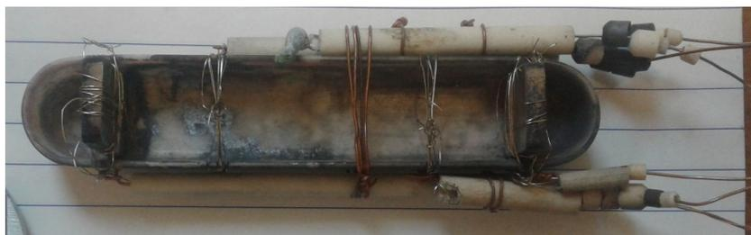
Figure 30: 4-probe crucible for NaSi conductivity
