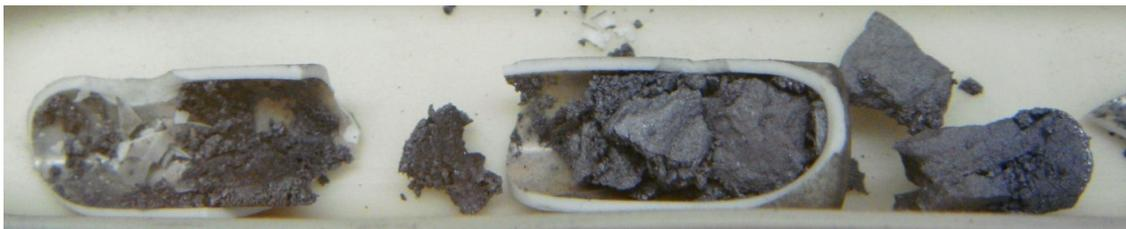
Figure 62: Sample A9, post autoclave heating at 875°C.
