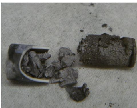
Figure 63: Sample A10, post autoclave heating at 900°C.
