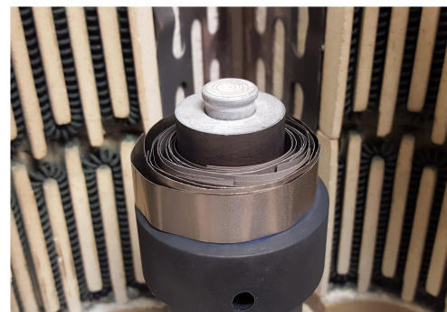
(b) Assembly of sample holder (top) and assembled sample holder with Ti foil (bottom).
