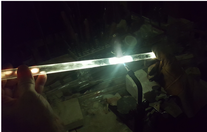
Figure 3.7: Glassblowing process for fabricating ampoules. Left: constricting a quartz tube containing samples before evacuation. Right: collapsing the constriction with the tube under a \sim 10^{-4} Torr vacuum. These images were taken through one of the lenses of a pair of glassblowing glasses.
