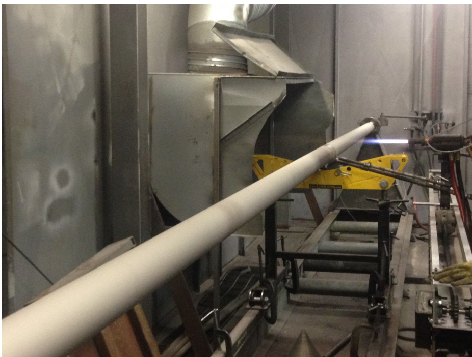
Figure 2.21: HVOF spraying of a tube or shaft. The flame that carries metal particles can be seen exiting the spray gun. In contrast, there is no flame in the cold spray process, but only an invisible stream of particles. [96]
