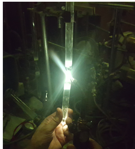
Figure 3.7: Glassblowing process for fabricating ampoules. Left: constricting a quartz tube containing samples before evacuation. Right: collapsing the constriction with the tube under a \sim 10^{-4} Torr vacuum. These images were taken through one of the lenses of a pair of glassblowing glasses.
