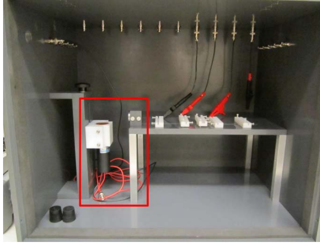
Figure 3-12, Light tight enclosure for scintillation detector experiments. BNC connectors are used to transmit signal and power across the box. The white stages are made of Delrin and aligned along the track in the platform, as is the adjustable PMT holder (red box).
