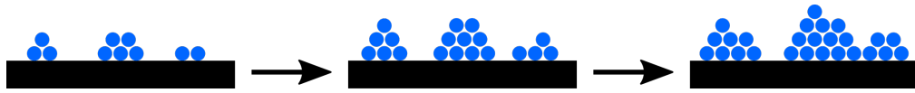
Figure 2.11: Volmer-Weber nucleation mechanism that forms 3D islands of irregular size which eventually cluster together. Typical for growth on amorphous substrates due to the inability for species to lattice match.
