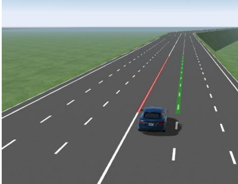
Fig.5.13. Detection of Lane Markings by Host Autonomous-capable EV.
