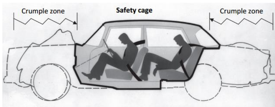
Figure 2.2: Schematic of the two major crash zones of a vehicle [8].
