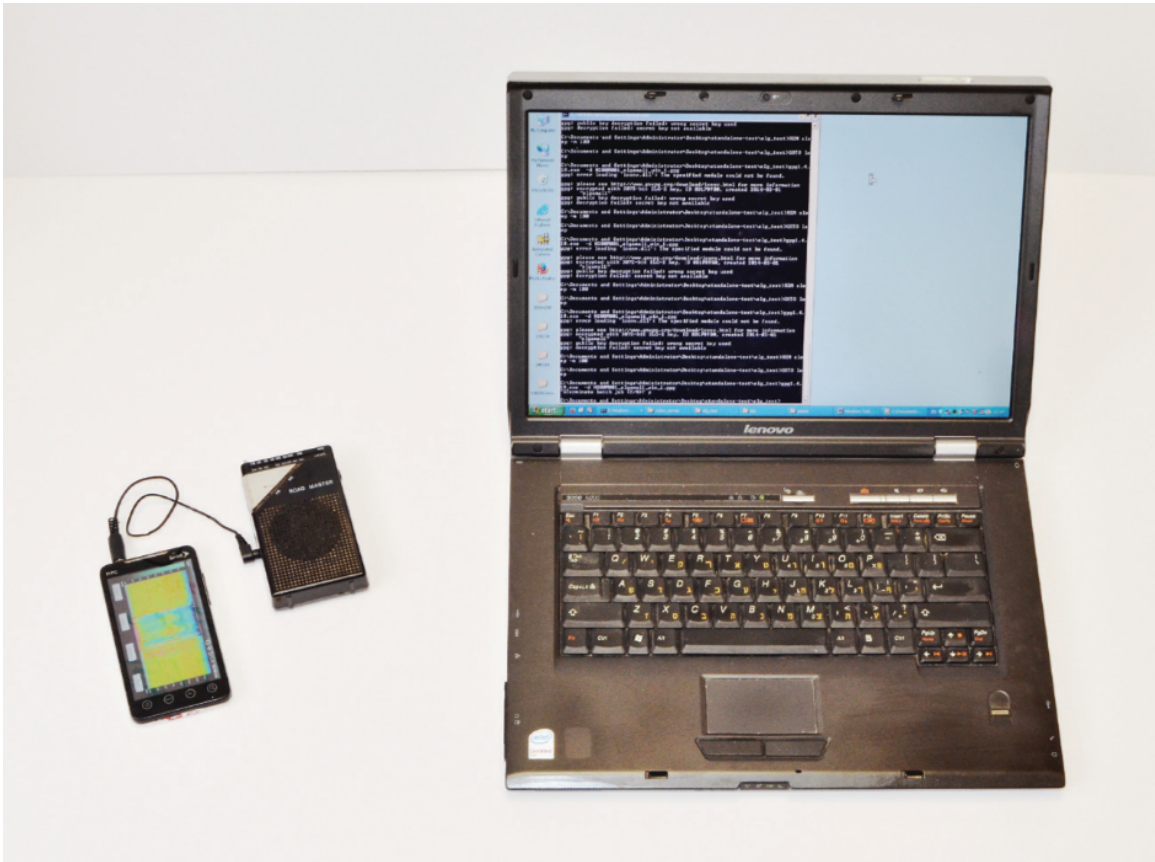
Figure 1.4: An electromagnetic attack using a consumer AM radio receiver placed near the targeted device and recorded by a smartphone [43].
