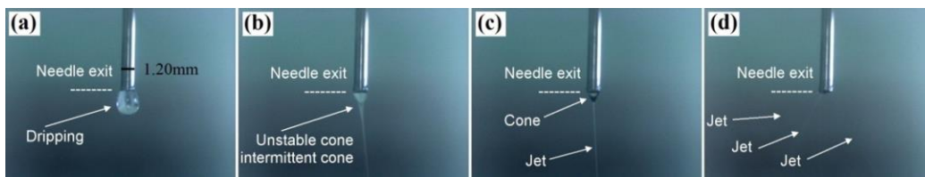
Figure 2.1: Different modes of EHD: (a) dripping mode, (b) unstable cone mode, (c) stable cone/jet mode, (d) multijet mode. Adapted from [162]
