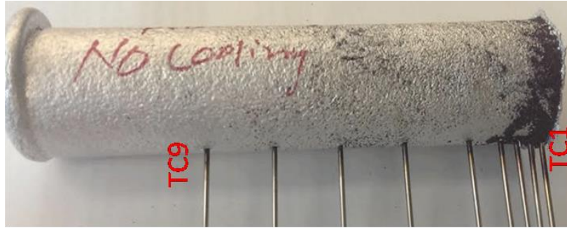
Figure 3.3 As-cast sample showing thermocouples embedded
