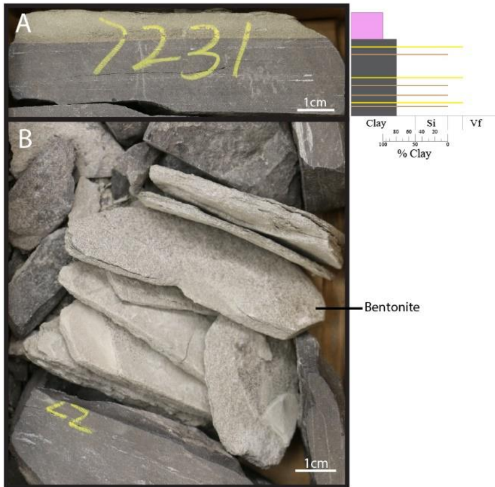
Fig. 19. Photographs highlighting bentonite ash layers A). A bentonite ash layer, sharply overlying silty and sandy parallel planar laminated mudstone at 7231.00ft. B). Fractured pieces of bentonite found at 7322.55ft.
