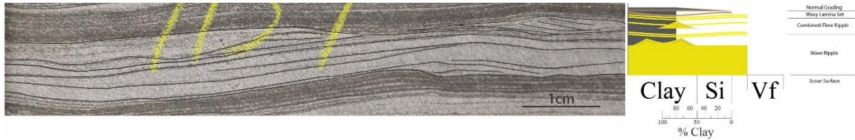
Fig. 22. Example and line drawing of a tempestite deposit showing from an upward succession a basal wave scour, wave rippled laminations, combined-flow ripple laminations, wavy lamina set, and normally graded lamination. Taken from 7137ft.
