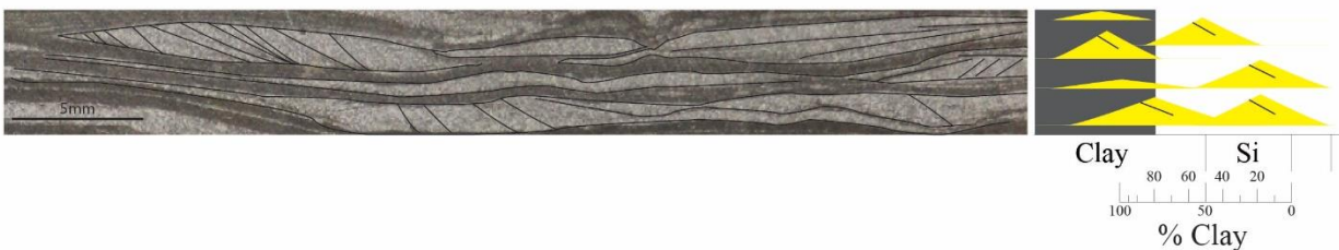
Fig. 26. Example and line drawing of a tidal wavy bedding. Clear bipolar current ripple cross laminations can be seen. Taken from 7134.80'.
