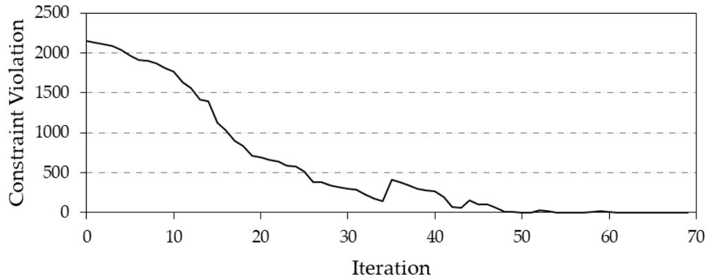
Figure 5.15: Constraint violation versus iteration number for solving the 5 period model using the end of the decomposition (after 1 run of the decomposition) as the initial guess to nominal operation optimality. Solved using IPOPT at the default tolerance.
