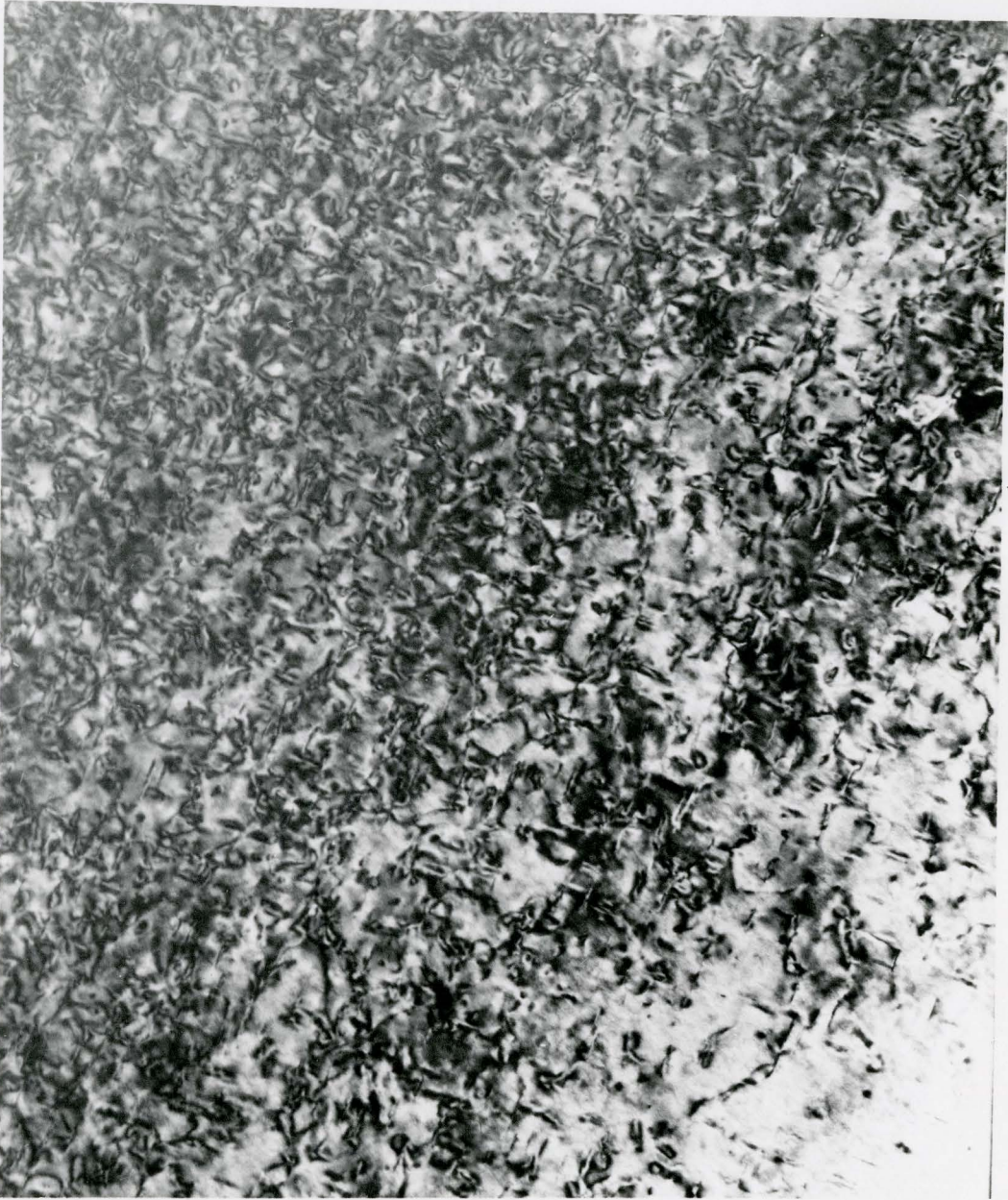
Fig. VI/33. Specimen from test number 16 showing \theta' precipitates with some dislocations.
