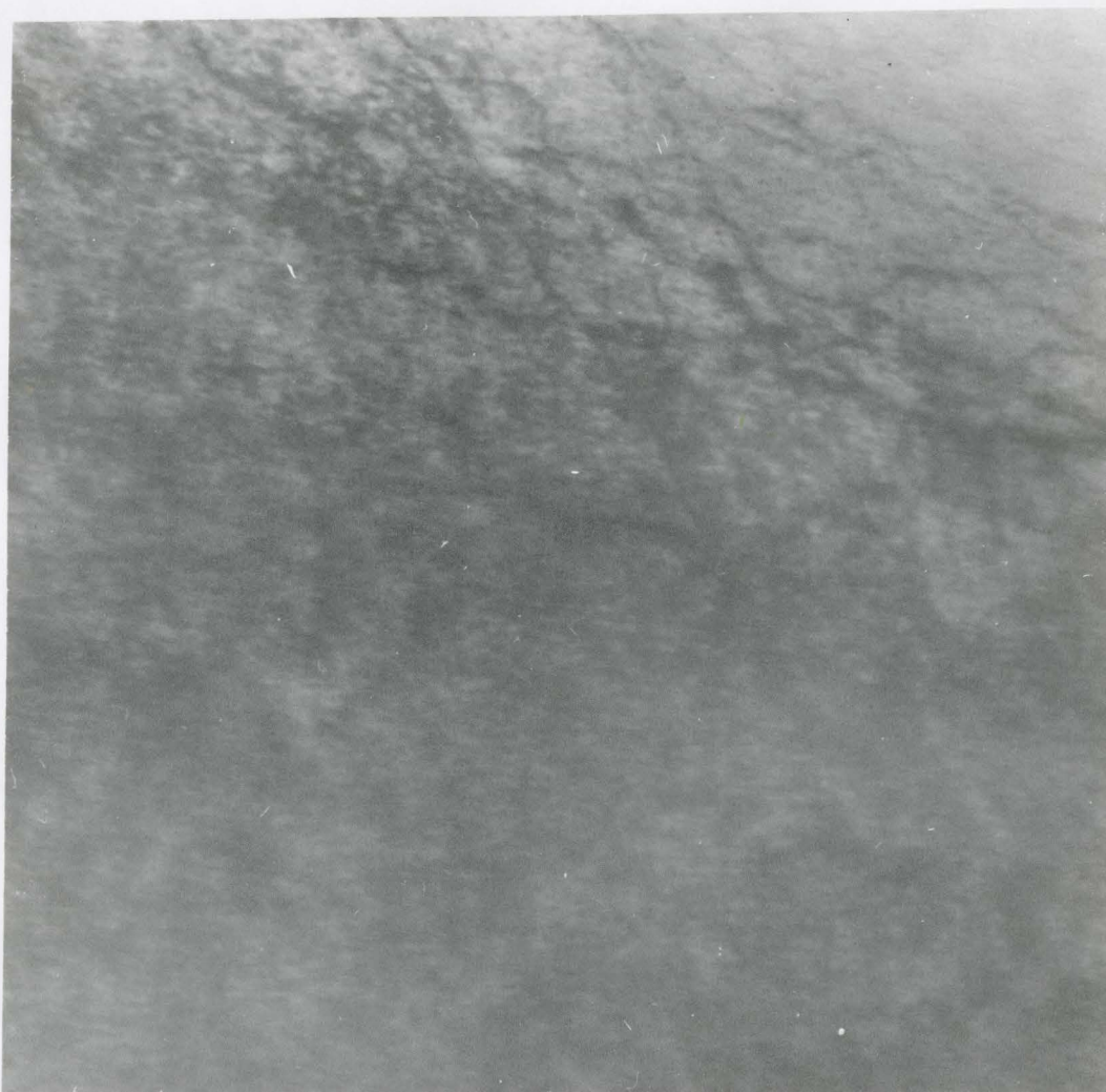
Fig. VI/29. Mottled background of GP zones with some dislocations. Test number 15.
