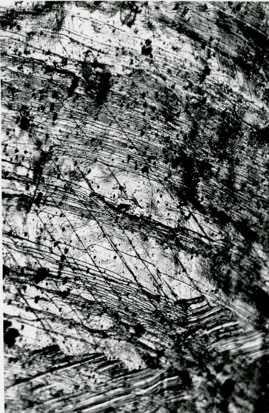
Fig. VI/25. Surface of a specimen containing \theta'' precipitates after fracture at room temperature. The area is near the fracture. Slip lines indicating cross-slip.
