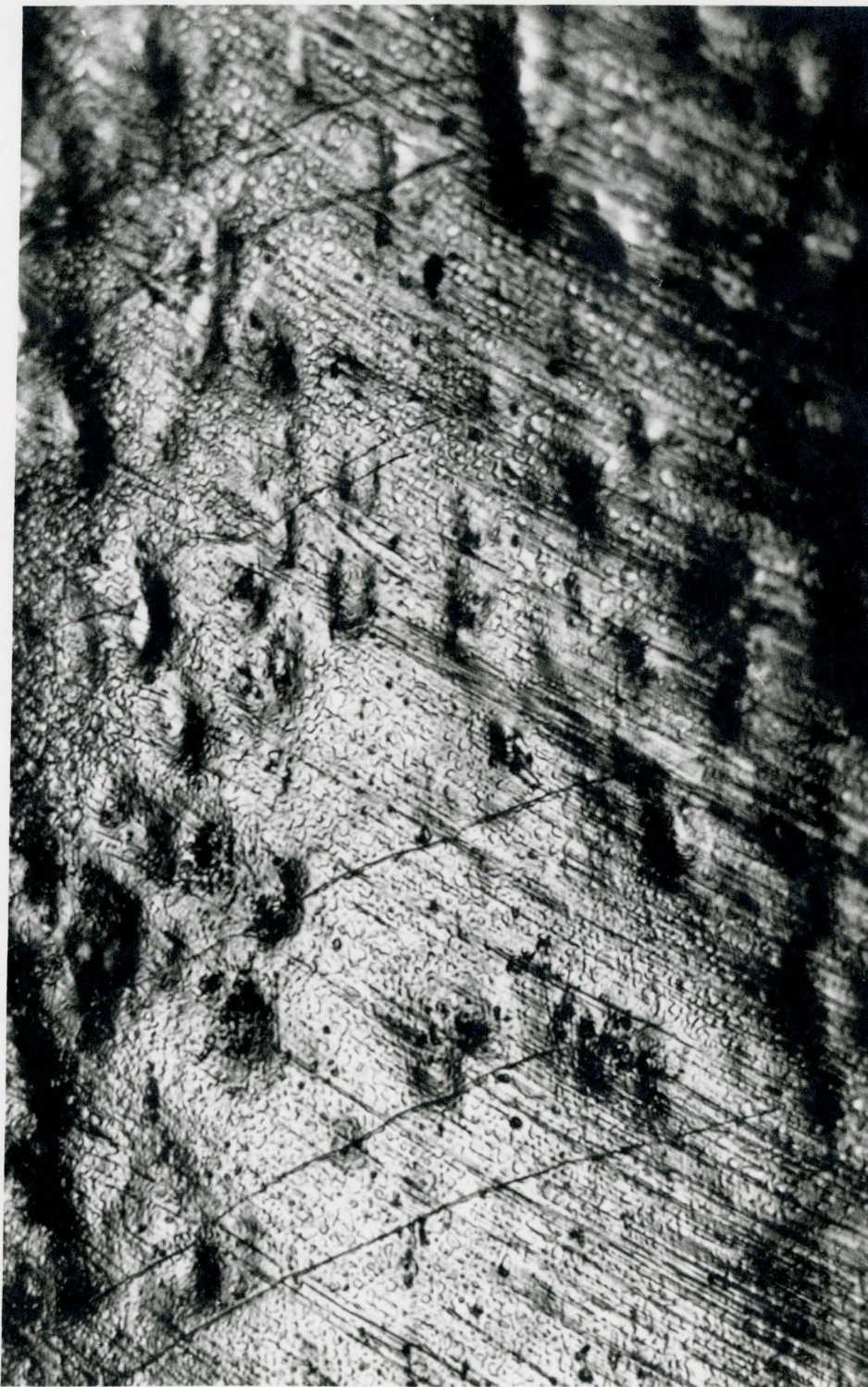
Fig. VI/23. Surface of a specimen containing GP zones after fracture at room temperature.
