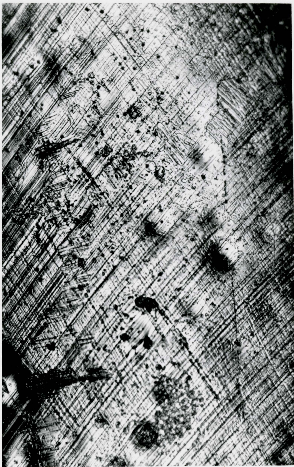
Fig. VI/24. Surface of a specimen containing \theta'' precipitates after fracture at room temperature.
