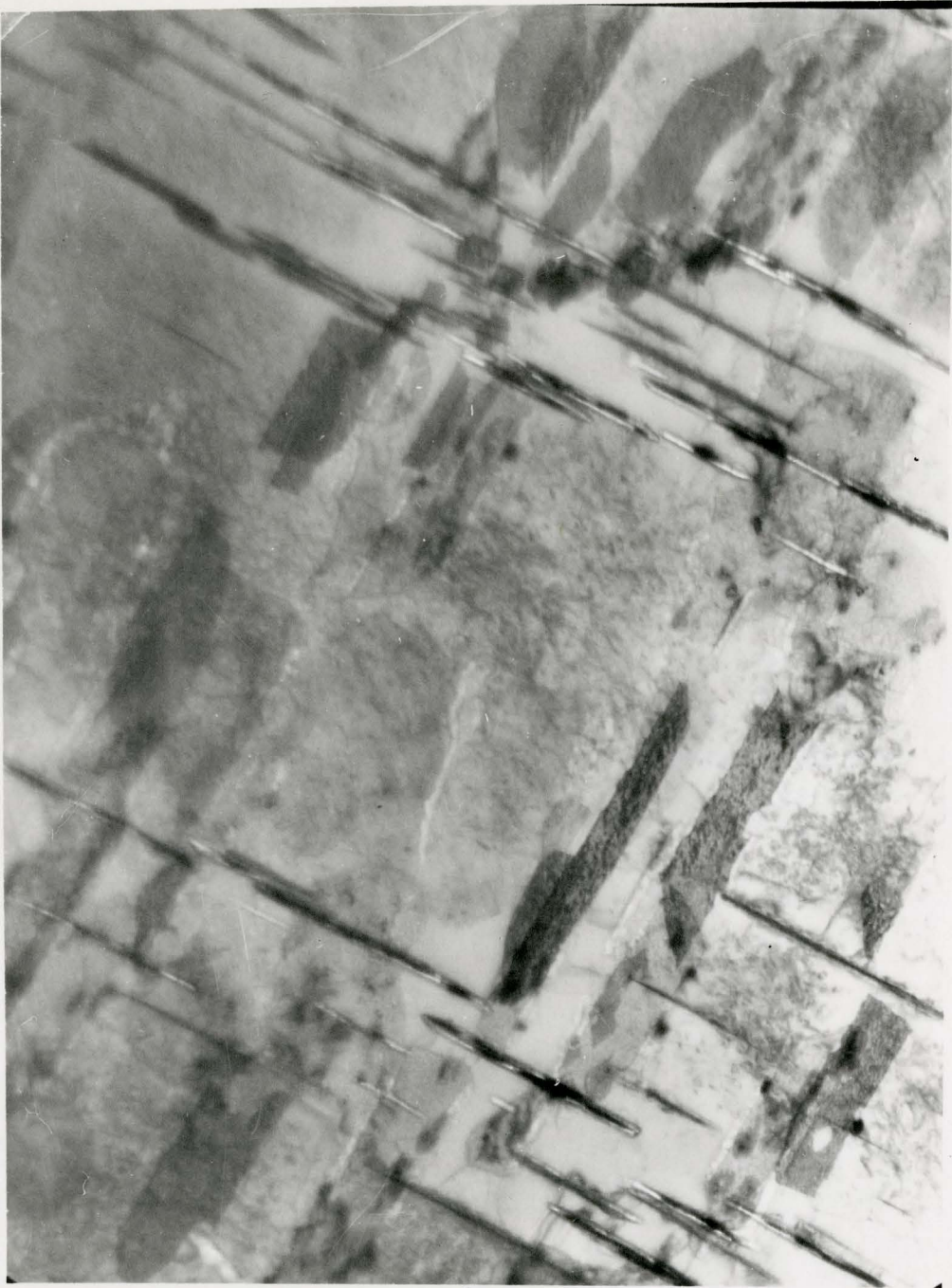
Fig. VI/37. \theta' precipitates and dislocation arrangement as it appears in specimen 8 after deformation.
