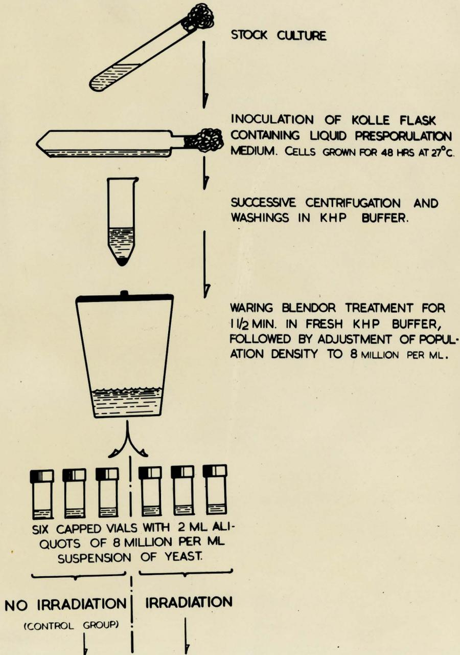
FIGURE 1 a . FLOW DIAGRAM OF EXPERIMENTAL PROCEDURE . This diagram summarizes the procedure up to and including the irradiation. See text for step by step description of the experimental procedure.
