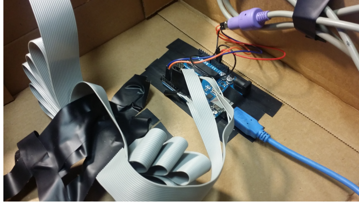
Figure 3.9: Arduino-controlled trigger system. The colored wires belong to the keyboard whereas the gray ribbon wires plug into the BioSemi ActiveTwo's trigger input (triggers are labels inserted into the system from an external device)
