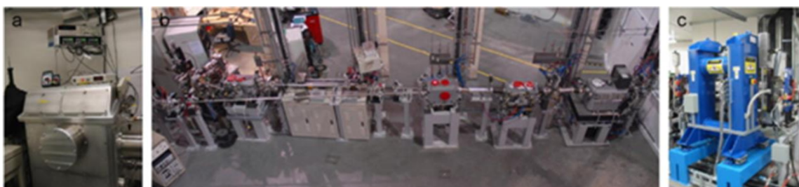
Figure 1.8 SM beam line photos: (a) STXM; (b) SM beamline. SR light propagates from right to the left; (c) Elliptically polarizing undulator (EPU). (reproduced with permission from (Kaznatcheev et al. 2007) Elsevier)
