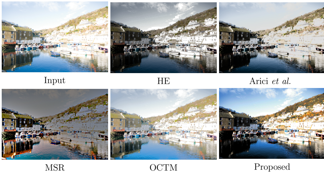
Figure 3.9: Results of enhancement algorithms on poor contrast images. The presented algorithms include: HE, modified HE by Arici et al. [3], multiscale Retinex algorithm, OCTM [72] and the proposed method.
