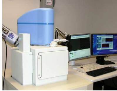
Figure 4.21: JOEL6610LV SEM/EDX system used in the characterization of the microstructure and chemical composition of the phases.
