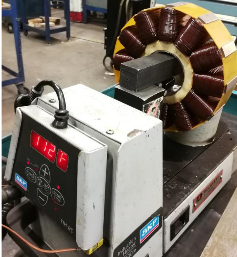
Fig. 7.14 Stator heating using induction heater (12/16 prototype)
