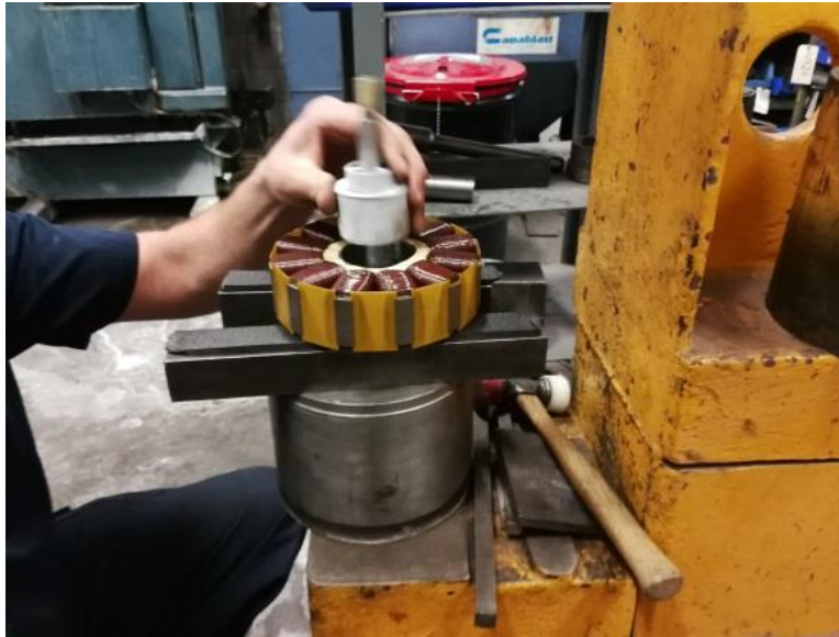
Fig. 7.16 Shaft insertion procedure
