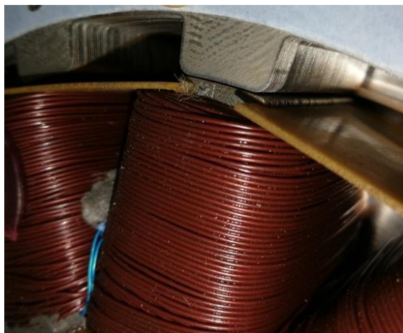
Fig. 7.20 Axial stack alignment (12/16 prototype)
