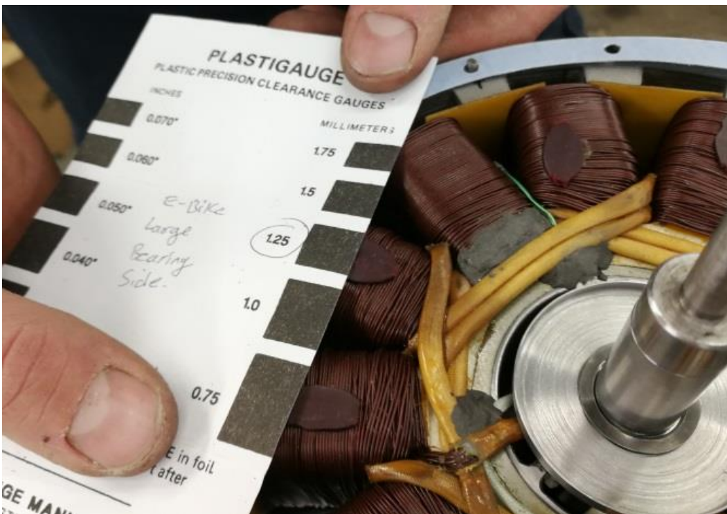
Fig. 7.21 Plastigauge testing of internal clearances (side “A” shown – side “B” circled)
