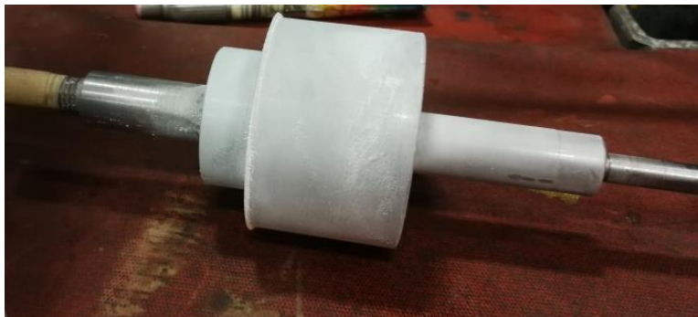
Fig. 7.15 Shaft cooling before insertion (12/16 prototype)
