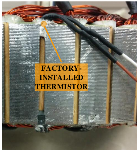
Fig. 5.6 Factory-installed thermistor location
