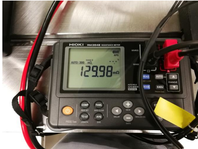
Fig. 7.27 Phase resistance measurement
