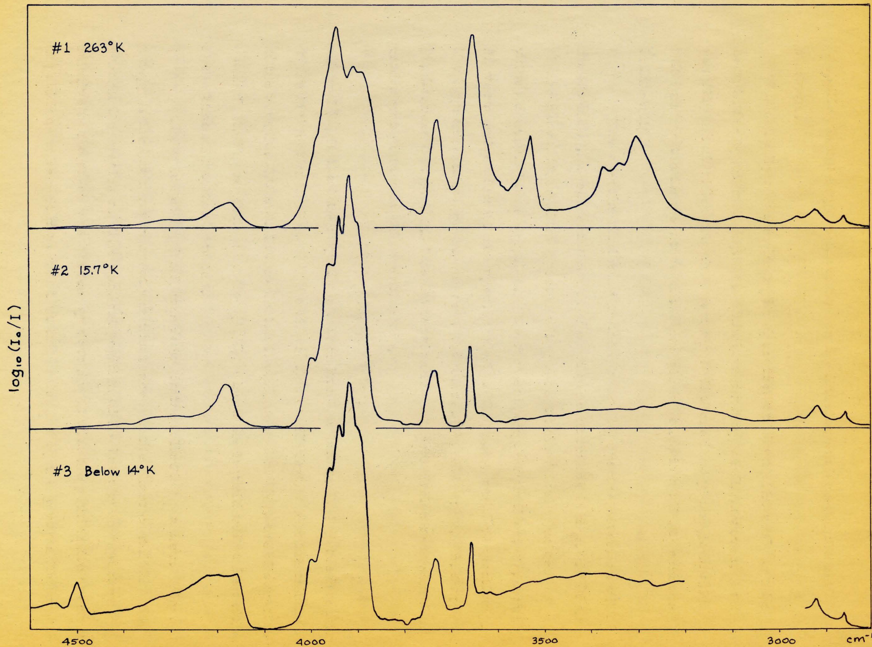
Fig.13. Infrared Absorption Profiles of Portlandite at Various Temperatures ( \varphi = 30^\circ , and Radiation Unpolarized)
