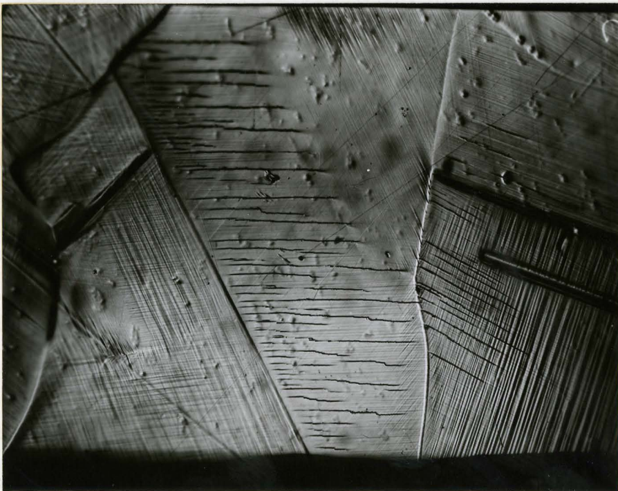
Fig. 12 High strain amplitude reverse bending - 1 cycle. X150
