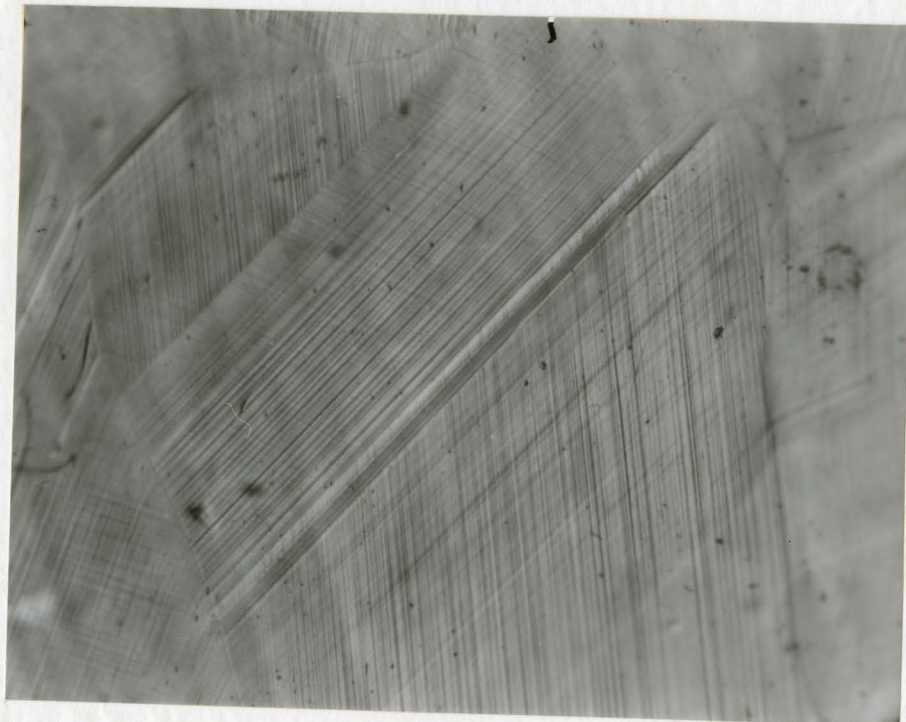
Fig. 11 Ordered \text{Cu}_3\text{Au} - deformed by low strain amplitude fatigue. X150
