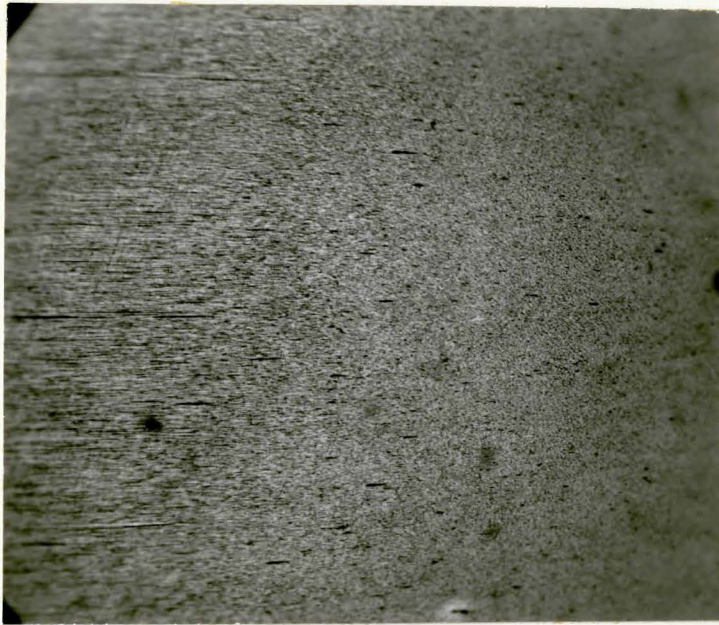
Figure 34. Section parallel to specimen axis on tensile specimen with tensile neck on right. Specimen axis horizontal. 45 x
