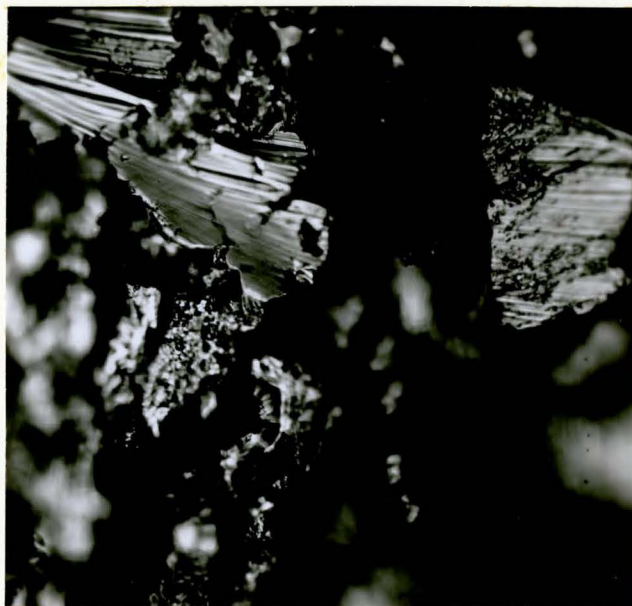
Figure 26. Optical micrograph of fatigue fracture surface. 460 x
