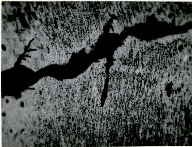
Figure 30. Section through fatigue crack. 350 x Specimen axis vertical.
