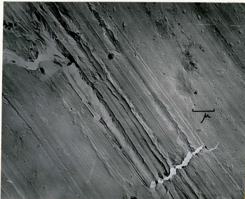
Figure 19. Electron fractograph of fatigue fracture surface.
