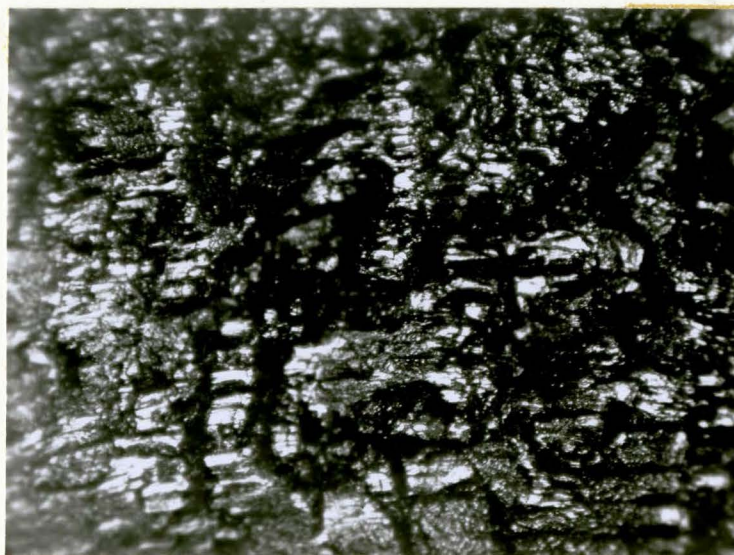
Figure 22. Fatigue cracks on specimen surface. 120 x Specimen axis horizontal.
