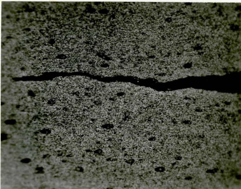
Figure 35. Section through root of axial crack. 460 x Specimen axis horizontal.
