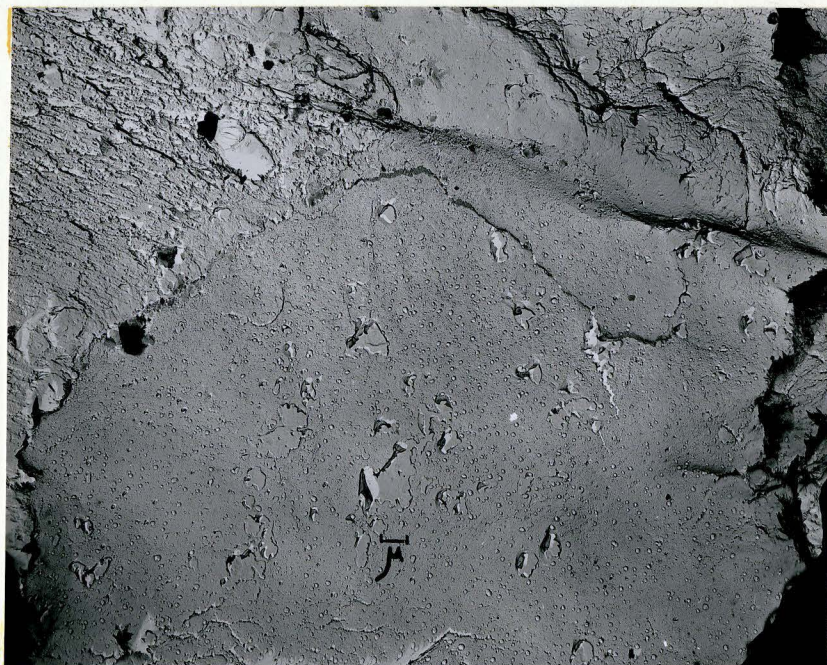
Figure 17. Electron fractograph of fatigue fracture surface.
