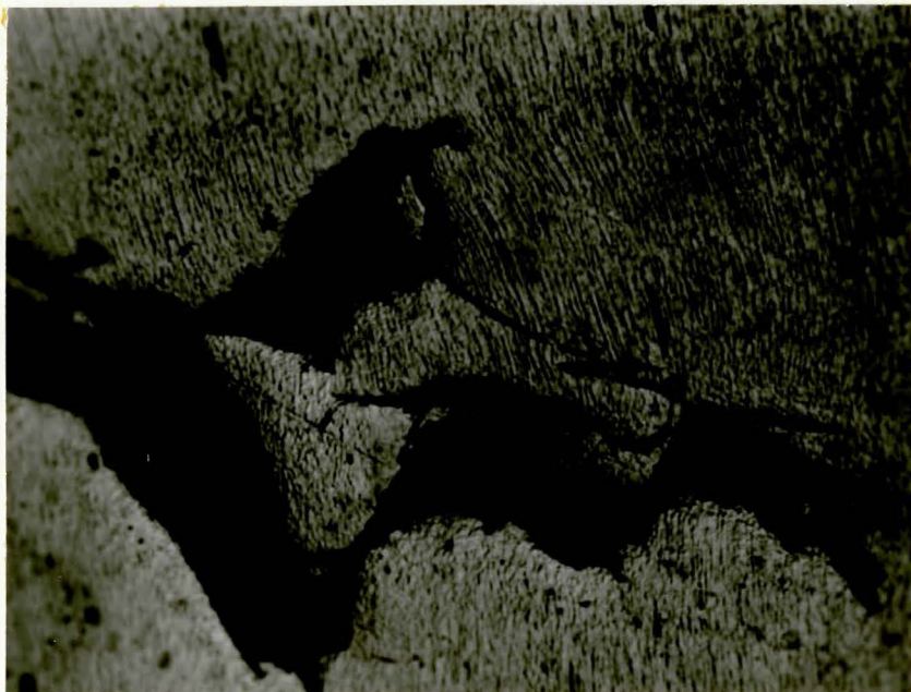
Figure 30. Section through fatigue crack. 350 x Specimen axis vertical.
